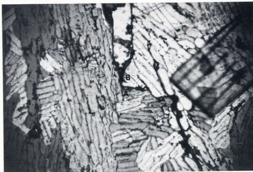
Fig. 15. Crack-tip region in specimen RT9 at 5 times magnification (scale gradations are 1 mm).
