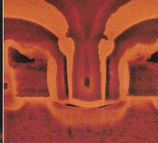
Integrated circuit with multiple film layers.
