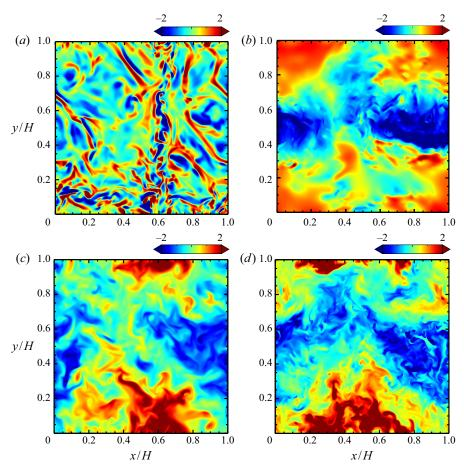
Figure 9. The instantaneous convection heat flux wT on (a,b) the near-wall plane  $z/\delta \approx 1$  and (c,d) the midplane z/H = 1/2 at  $Ra = 10^9$ ; (a,c) the impermeable case  $\beta U = 0$  and (b,d) the supercritical permeable case  $\beta U = 3$ . The heat flux wT on the horizontal plane is normalised so that its mean and standard deviation may be zero and unity, respectively.
