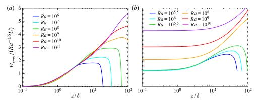
Figure 4. The RMS vertical velocity normalised by  $Ra^{-1/6}U$  as a function of  $z/\delta$ ; (a) the impermeable case  $\beta U=0$  and (b) the permeable case  $\beta U=3$ .
