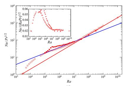
Figure 12. The Nusselt number Nu compensated by  $Pr^{1/2}$  as a function of the Rayleigh number Ra. The filled and open circles represent the present DNS data for Pr=7 and Pr=1 in the permeable case  $\beta U=3$ , respectively. The red and blue line indicate  $Nu \sim Pr^{1/2}Ra^{1/2}$  and  $Nu \sim Ra^{1/3}$ , respectively. The inset shows Nu compensated by  $(RaPr)^{1/2}$ .
