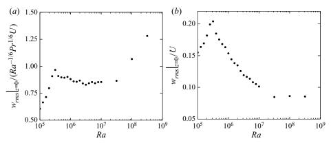
Figure 13. The RMS vertical velocity on the wall z = 0 normalised by (a)  $Ra^{-1/6}Pr^{1/6}U$  and (b) U in the permeable case  $\beta U = 3$  for Pr = 7.
