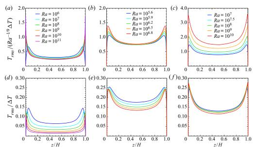
Figure 6. The RMS temperature normalised by (a-c)  $Ra^{-1/9}\Delta T$  and (d-f)  $\Delta T$ ; (a,d) the impermeable case  $\beta U=0$ , (b,e) the subcritical permeable case  $\beta U=3$  at  $10^{5.6}\leqslant Ra\leqslant 10^{6.8}$  and (c,f) the supercritical permeable case  $\beta U=3$  at  $10^7\leqslant Ra\leqslant 10^{10}$ .
