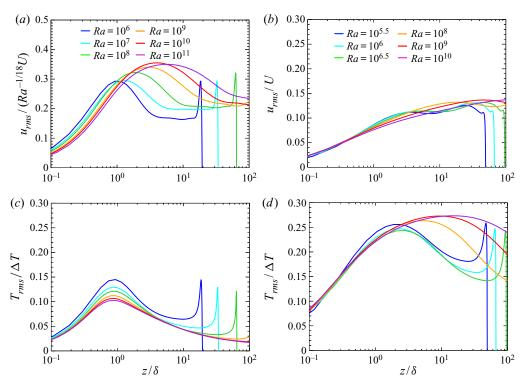
Figure 7. The near-wall RMS velocity and temperature as a function of  $z/\delta$ . (a,b) The RMS horizontal velocity normalised by  $Ra^{-1/18}U$  and U and (c,d) the RMS temperature normalised by  $\Delta T$ ; (a,c) the impermeable case  $\beta U=0$  and (b,d) the permeable case  $\beta U=3$ .
