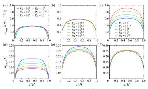
Figure 5. The RMS vertical velocity normalised by (a-c)  $Ra^{-1/18}U$  and (d-f) U; (a,d) the impermeable case  $\beta U=0$ , (b,e) the subcritical permeable case  $\beta U=3$  at  $10^{5.6} \leqslant Ra \leqslant 10^{6.8}$  and (c,f) the supercritical permeable case  $\beta U=3$  at  $10^7 \leqslant Ra \leqslant 10^{10}$ .
