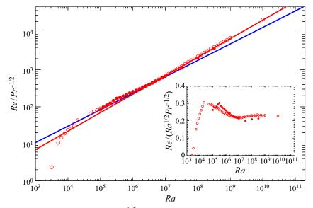
Figure 14. The Reynolds number  $Re = \langle w^2 \rangle_{xyzl}^{1/2} H/v$  compensated by  $Pr^{-1/2}$  as a function of the Rayleigh number Ra. The filled and open circles represent the present DNS data for Pr=7 and Pr=1 in the permeable case  $\beta U=3$ , respectively. The red and blue line indicate  $Re \sim Pr^{-1/2}Ra^{1/2}$  and  $Re \sim Pr^{-2/3}Ra^{4/9}$ , respectively. The inset shows Re compensated by  $Ra^{1/2}Pr^{-1/2}$ .
