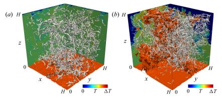
Figure 8. Instantaneous thermal and vortical structures in (a) the impermeable case  $\beta U=0$  and (b) the supercritical permeable case  $\beta U=3$  at  $Ra=10^9$ . The orange and grey objects, respectively, represent the isosurfaces of the temperature  $T/\Delta T=0.7$  and of the second invariant of the velocity gradient tensor, (a)  $Q/(v^2/H^4)=8\times 10^{10}$  and (b)  $Q/(v^2/H^4)=4.8\times 10^{11}$ . The colour indicates the temperature distribution on the planes x=0 and y=H.
