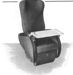
Six types of aircraft seating may be inspected at our Stand No. 34 Grande Nef at the International Aeronautical show in Paris. The seat illustrated is the Mark 33, a fully reclining single chair for long-range luxury aircraft. It incorporates the well-known B.O.A.C. adjustment principle, and can be fitted with tables and other accessories.
