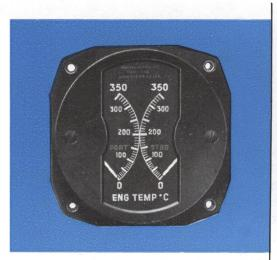
Model S. 128. Dual Engine Temperature Indicator, comprising two Millivoltmeters of 100° scale housed in large-size S.A.E. case. For use in conjunction with copper/constantan, iron/constantan, or chrome/alumel thermocouples.
