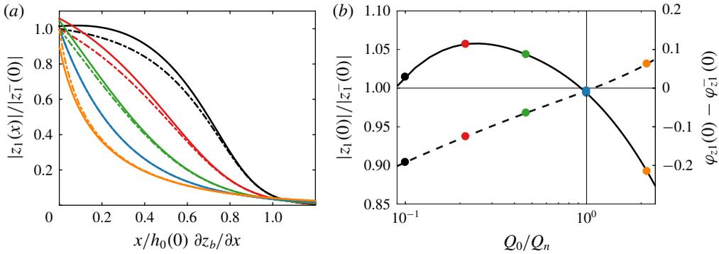
FIGURE 12. (Colour online) (a) Admittance of the combined incoming and reflected waves ( $|z_1(x)|/|z_1^-(0)|$ , solid) and only of the upstream travelling wave ( $|z_1^-(x)|/|z_1^-(0)|$ , dash-dotted) along the river. (b) amplitude (solid) and phase (dashed) of the combined wave with respect to the incoming wave at the river mouth, depending on the river discharge. Scenarios as in figure 8.
