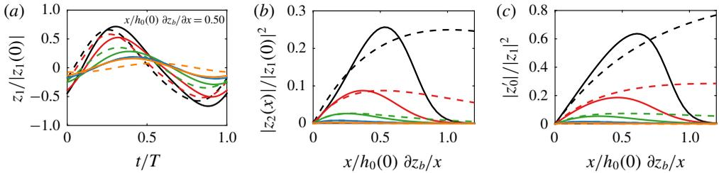
FIGURE 14. (Colour online) (a) At a station, water level variation over a tidal cycle for  $z_1(0) = 0.1h_0(0)$ ; (b) along river amplitude of the even overtide; (c) along river subtidal water level set-up; solid lines show the tide in a backwater affected river, and dashed lines show the prediction of the tide when the backwater is neglected; scenarios as in figure 8.
