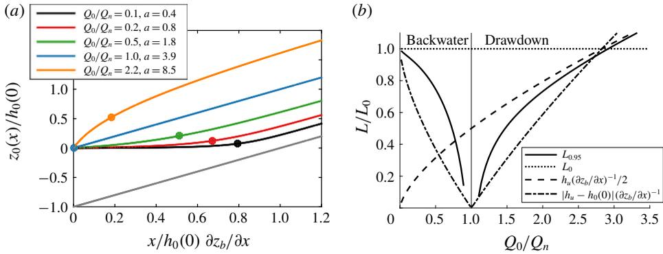
FIGURE 7. (Colour online) (a) Tidally averaged water level along the river, where the backwater drawdown lengths are indicated by dots; (b) backwater and drawdown length  $L$  for various states of river flow, defined as the distance to point where water depth deviates no more than 5% ( $L_{95}$ ) and approximated by simplified relations.
