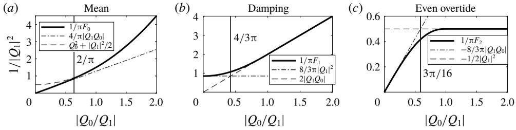
FIGURE 5. Magnitudes of the frequency components of the friction term ((3.8a)–(3.8c), bold), depending on the relative strength of river and tidal flow ( $|Q_0|/|Q_1|$ ), as well as their low flow asymptotes ( $|Q_0|/|Q_1| \rightarrow 0$ , dash-dotted) and high flow asymptotes ( $|Q_0|/|Q_1| \rightarrow \infty$ , dashed). Note that the discharge scale is identical to the velocity scale as  $|u_0|/|u_1| = |Q_0|/|Q_1|$ .
