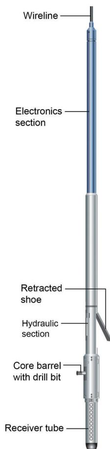
**Fig. 8.** Schlumberger Ltd mechanical side-wall coring tool (Schlumberger, 2004).
