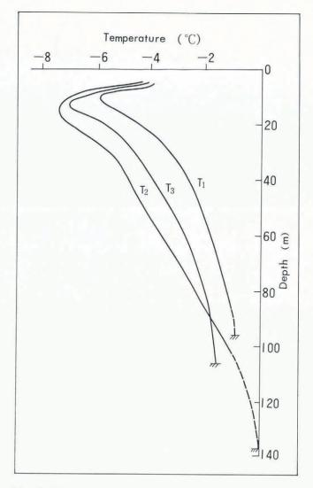
Fig. 5. Temperature profiles measured on Urumqi Glacier No. 1 on 27 September 1986. The dotted lines are extrapolated (after Cai, unpublished).
