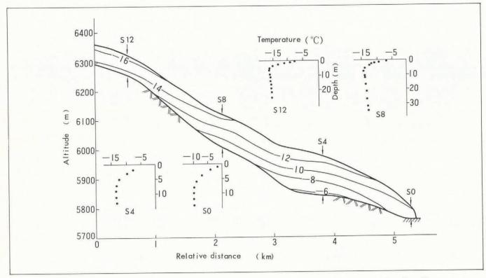
Fig. 2. Two-dimensional temperature distribution in a longitudinal profile of Chongce Ice Cap. West Kunlun Mountains (after Zhou and Han, 1990).
