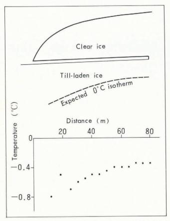
Fig. 6. Section through the tunnel in Urumqi Glacier No. 1 with its temperature profile measured during excavation in September-October 1988 (by courtesy of Zhou Tao).
