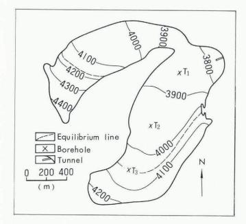
Fig. 4. A map showing the locations of holes for temperature measurement and the artificial tunnel in Urumqi Glacier No. 1.
