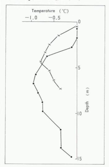
Fig. 7. Temperature profiles of two temperate-type glaciers. ×, upper part of the ablation area (4600 m) on Glacier No. 1, Baishuihe, 11 July 1982; -, middle part of the ablation area (4540 m) on Dagongba Glacier, 30 September 1982. The glacier surface at the time of measurement is taken as the origin of the depth coordinate (by courtesy of Wang Lilun).
