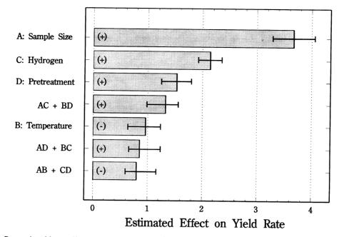
Fig. 2. Pareto plot of factor effects on percent yield rate from factorial-designed experiment. The sample size effect is most significant. Error bars are ranges in factor effect values generated through the Monte Carlo technique (see text).
