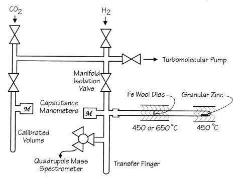
Fig. 1. Carbon dioxide reduction system. Thermocouple-controlled furnaces maintain temperatures of iron wool catalyst and zinc. Gases are sampled in 525 mm<sup>3</sup> aliquots for mass spectrometry by a glass 120° V-bore stopcock valve (see text).
