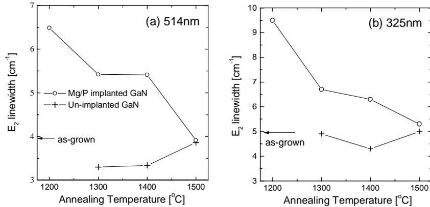
**Figure 1.**  $E_2$  phonon linewidth of ion-implanted and of un-implanted GaN films determined (a) under 514nm- and (b) under 325nm-excitation. The  $E_2$  phonon linewidth is a measure for the crystalline quality of the GaN.
