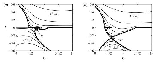
FIGURE 8. Spatial branches  $k^{\pm}(\omega')$  of the Doppler-shifted unconfined dispersion relation (4.6) and saddle point  $k^*$  resulting from the pinching of these branches as  $\omega'_i$  decreases, for (a) p = 0.3,  $v_g = -1.62$  and (b) p = 0.35,  $v_g = -2.03$ . In both cases, these critical values of  $v_g$  give  $\omega'_i(k^*) = \sigma(v_g) = 0$  and hence correspond to  $v_g^-$ .
