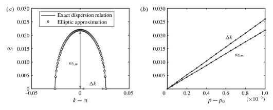
FIGURE 9. Self-similar behaviour of the dispersion relation in a narrow range of p around the stable value  $p_0$ . (a) Temporal growth rate  $\omega_i(k)$  evaluated at  $p = p_0 + 0.001$ , together with its elliptic approximation  $\omega_i^e(k)$  and the definitions of  $\omega_{i,m}$  and  $\Delta k$ . (b) Linear dependency of  $\omega_{i,m}$  and  $\Delta k$  on p as the latter approaches  $p_0$ .
