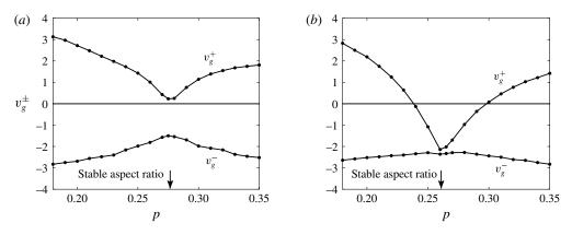
FIGURE 11. Leading- and trailing-edge velocities  $v_g^{\pm}$  of the impulse response wave packet generated by a localized initial perturbation versus aspect ratio p, for two values of the confinement ratio, (a) q = 1.6 and (b) q = 1.2. The velocities given by the numerical simulations are represented with dots and joined by straight lines.
