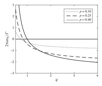
FIGURE 2. Non-dimensional self-induced velocity  $2\pi av_0/\Gamma$  of the vortex street versus confinement ratio q, for different values of the aspect ratio p. As q increases, the self-induced velocity tends to its unconfined value of -0.9557 (p=0.10), -2.0602 (p=0.25) and -2.6708 (p=0.40).
