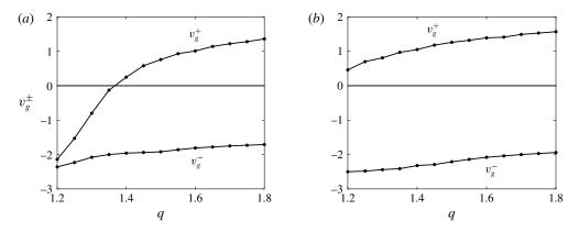
FIGURE 12. Leading- and trailing-edge velocities  $v_g^{\pm}$  of the impulse response wave packet generated by a localized initial perturbation versus confinement ratio q, for two values of the aspect ratio, (a) p = 0.26 and (b) p = 0.31. The velocities given by the numerical simulations are represented with dots and joined by straight lines.
