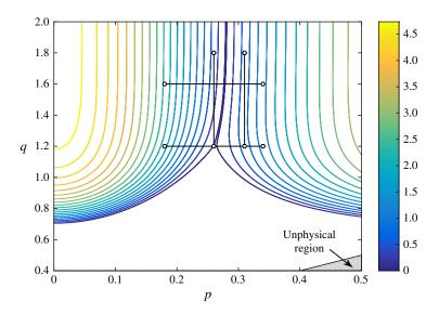
FIGURE 4. (Colour online) Temporal dispersion relation. Isolines of the growth rate of the most unstable wavenumber versus aspect ratio p and confinement ratio q. The black lines indicate the range of parameter values under which the spatio-temporal characteristics of the impulse response of the vortex street is evaluated in figures 11 and 12.
