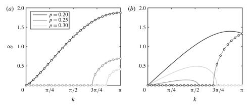
FIGURE 3. Temporal dispersion relation. Growth rate  $\omega_i$  of the symmetric (continuous line) and antisymmetric (dotted line with circles) modes versus wavenumber k, for different aspect ratios p and (a) q = 20, i.e. almost no confinement, and (b) q = 1.2, i.e. strong confinement. The growth rate of antisymmetric perturbations of wavenumber  $2\pi - k$  is equivalent to that of symmetric perturbations of wavenumber k and vice-versa.
