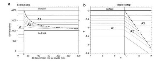
**Fig. 2.** Isochrones over a step change in bedrock elevation at  $x = x_1$  (corresponding to  $\pi = \pi_1$ ), marked by a thick grey vertical line. Ice is in plug flow. (a) (x, z)-coordinate system. (b)  $(\pi, \theta)$ -coordinate system. In both panels, thin black lines (plain and dot–dashed) are isochronous layers, and the thick dashed line is the trajectory of a particle deposited immediately upstream of the bedrock step (see section 4.1 for a complete description of the zones).
