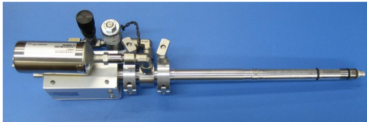
Fig. 1: Picture of the Oxygen Radical Source (ORS) on a TEM Holder. The RF electrode is on the right hand side near where a TEM sample would normally be. The valve assembly, pressure gauge and impedance match are on the left hand side of the picture.
