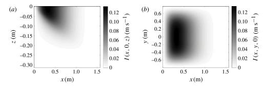
FIGURE 3. Impulse due to the body force parametrizing a breaking event. The plot on the left shows the impulse in the (x, z) plane at y = 0 while the plot on the right shows the impulse in the (x, y) plane at z = 0; based on forcing given in SMM2004, which is in the  $\hat{x}$  direction.
