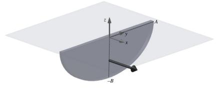
FIGURE 5. Sketch of a thin elliptical half disc of major axis length 2A and minor axis length 2B being forced from rest to a velocity  $U\hat{x}$  through a fluid with surface at z = 0. Here z < 0 corresponds to water while z > 0 corresponds to air.
