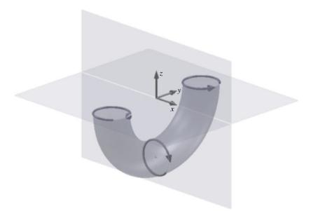
FIGURE 4. Description, proposed by Peregrine (1999), of the topological shape (a half vortex ring) of the flow shortly after a breaking event. The surface of the torus denotes the vortex filament and the arrows indicate the direction of the velocity.
