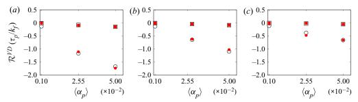
Figure 7. Viscous diffusion Eulerian–Lagrangian results ( $\circ$ , streamwise component and  $\square$ , cross-stream components) and model prediction (( $\bullet$ , red), streamwise component and ( $\blacksquare$ , red), cross-stream components). Model corresponds to (4.8) and results from  $\lambda = 0.2$ . The associated model error is 0.07: (a) Ar = 1.8; (b) Ar = 5.4; and (c) Ar = 18.0.
