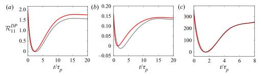
Figure 9. Temporal evolution of drag production obtained from the learned model 4.5 (——, very thick solid, red) and Euler–Lagrange data (—-, very thick dotted, black) for CIT after gravity is reversed instantaneously: (a) Ar,  $\langle \alpha_p \rangle = (1.8, 0.0255)$ ; (b) Ar,  $\langle \alpha_p \rangle = (5.4, 0.001)$ ; and (c) Ar,  $\langle \alpha_p \rangle = (18, 0.05)$ .
