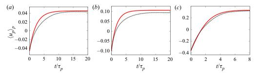
Figure 10. Temporal evolution of mean particle settling velocity obtained from the multiphase RANS equations (——, very thick solid, red) and Euler–Lagrange data (—, very thick dotted, black) for CIT after gravity is reversed instantaneously: (a) Ar,  $\langle \alpha_p \rangle = (1.8, 0.0255)$ ; (b) Ar,  $\langle \alpha_p \rangle = (5.4, 0.001)$ ; and (c) Ar,  $\langle \alpha_p \rangle = (18, 0.05)$ .
