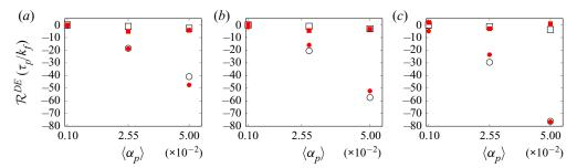
Figure 8. Drag exchange Eulerian–Lagrangian results ( $\circ$ , streamwise component and  $\square$ , cross-stream components) and model prediction (( $\bullet$ , red), streamwise component and ( $\blacksquare$ , red), cross-stream components). Model corresponds to (4.9) and results from  $\lambda = 0.006$ . The associated model error is 0.15: (a) Ar = 1.8; (b) Ar = 5.4; and (c) Ar = 18.0.
