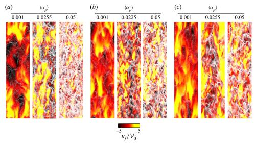
Figure 1. Instantaneous snapshots of fully developed CIT at statistical steady state. A slice at the centreline in the x-y plane is shown, with particle position (white) and normalized vertical fluid velocity  $u_f/\mathcal{V}_0$  (colour): (a) Ar = 1.80; (b) Ar = 5.40; and (c) Ar = 18.0.
