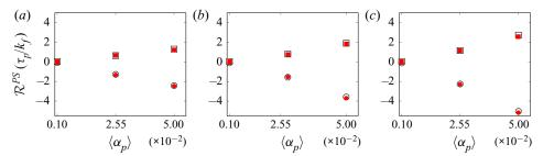
Figure 6. Pressure strain Eulerian–Lagrangian results ( $\circ$ , streamwise component and  $\square$ , cross-stream components) and model prediction (( $\bullet$ , red), streamwise component and ( $\blacksquare$ , red), cross-stream components). Model corresponds to (4.7) and results from  $\lambda = 0.3$ . The associated model error is 0.04: (a) Ar = 1.8; (b) Ar = 5.4; and (c) Ar = 18.0.
