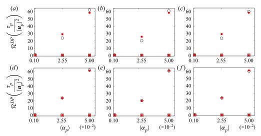
Figure 3. Drag production obtained from Eulerian–Lagrangian results ( $\square$ , cross-stream component and  $\circ$ , streamwise components) and model prediction (( $\blacksquare$ , red), cross-stream component and ( $\bullet$ , red), streamwise components). The model corresponds to (4.5) with  $\lambda = 0.01$ . The associated model error is  $\epsilon = 0.01$ . (a) Ar = 1.80; (b) Ar = 5.40; (c) Ar = 18.0; (d) Ar = 1.8; (e) Ar = 5.4; and (f) Ar = 18.0.
