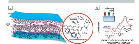
(a) Illustration of an electrolyte-free flexible electrochromic device of  $MV^{2+}$  graphene quantum dots (GQDs). (b) Cyclic voltammogram of 5 mM  $MV^{2+}$  at an indium-tin-oxide electrode in an aqueous solution containing 8 mg mL<sup>-1</sup> GQD (blue line) and 0.1 M KCl (red line) at a scan rate of 100 mVs<sup>-1</sup>. Inset: A depiction of a three-electrode cell composed of a working electrode (W), a counter electrode (C), and a reference electrode (R). Reproduced with permission.
