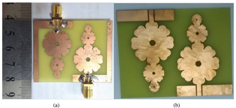
Fig. 9. Prototypes of the sunflower MIMO fractal antenna. (a) With ground side strip L . (b) Without ground side strip L .
