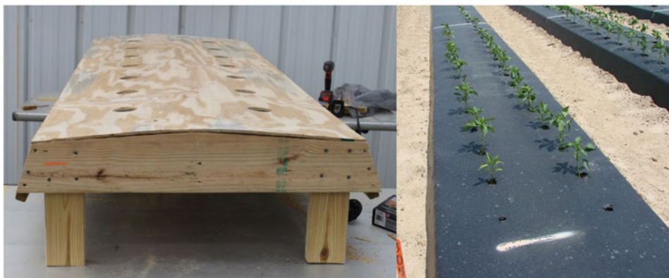
Figure 1. Left, Bed construction without carpet or plastic mulch covering. Design of the simulated bed was created to mimic a soil bed used in pepper production, including a slope of 6.7% from the middle to each side of the bed. Right, An actual field bed a . Phrase “in comparison to” seems redundant with “created to mimic.”
