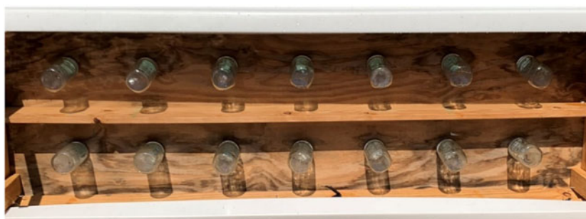
Figure 2. Bottom view of the constructed simulated bed with 14 glass jars attached representing transplant crop holes. Top row are jars 1–7 (left side of bed) and the bottom row are jars 8–14 (right side of bed), with jars being opposite going down the length of the bed (i.e., jars 1 and 8 are across from each other). Holes were spaced 30.5 cm apart from the center of one hole to the center of another and 20.3 cm from the center of one hole to the edge of the plywood.
