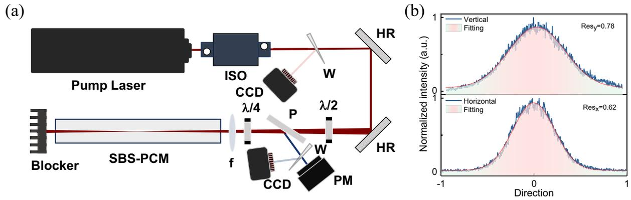
**Figure 1.** Experimental structure of the single-cell SBS-PCM. (a) Experimental setup. ISO, optical isolator; HR, highly reflective mirror; CCD, charge-coupled device-based beam quality analyzer;  $\lambda/2$ , half-wave plate. (b) Pump light distribution.
