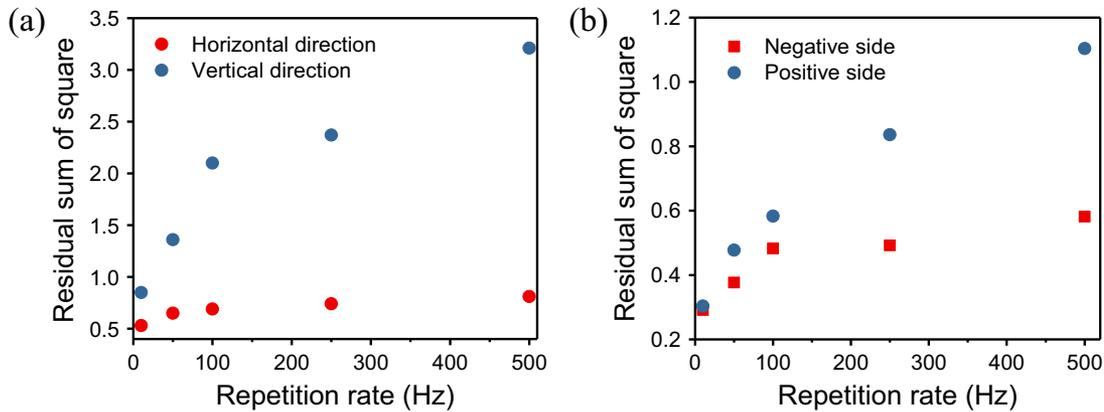
**Figure 5.** RSS of Gaussian fitting: (a) in the horizontal/vertical direction; (b) positive/negative side in the vertical direction.
