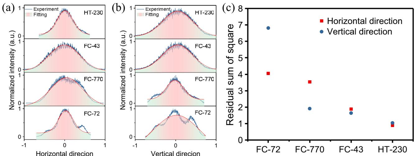
Figure 8. Gaussian fitting of different media: (a) horizontal direction; (b) vertical direction; (c) RSS of the fitting.
