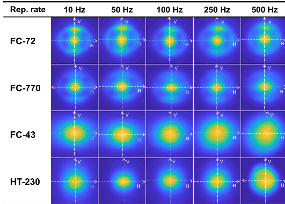
intense thermal convection occurred in FC-72 and FC-770, which had viscosities of less than 1, resulting in horizontal and vertical beam profile distortions. In contrast, little distortion was observed in FC-43 and HT-230, which had viscosities greater than 2. Higher-viscosity media effectively inhibited thermal convection, and the beam profiles closely resembled the  $TEM_{00}$  mode with Gaussian distribution. The discrepancies in the beam size displayed in Table 2 can
