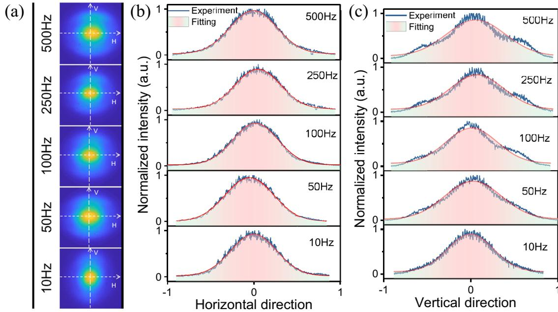
**Figure 4.** Beam profile at different repetition rates. (a) Beam profile. (b) Fitting in the horizontal direction. (c) Fitting in the vertical direction.
