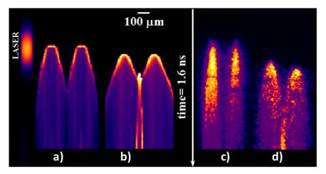
Figure 10. The temperature of the rear side obtained in 2D MULTI simulation for: (a)  $10 \mu m Al$ ; (b)  $10 \mu m Al + 50 mg/cm^3$  foam. For these simulations, we used a laser pulse with spatial flat-top profile and a Gaussian time profile, duration 300 ps (FWHM), wavelength 0.44  $\mu m$  (simulations with Gaussian spatial profile yield the same results). (c) and (d) Experimental rear-side self-emission streak images from Figure 2 (shots 30142 and 30147).
