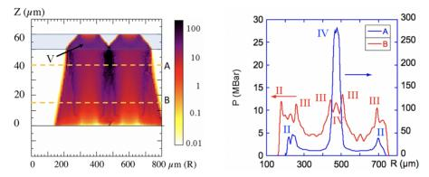
**Figure 14.** Time t = 0.52 ns: (left) hydro-simulations (as in Figure 11 but rotated by 90°); (right) pressure profiles at z = 18 and 45  $\mu$ m (dashed lines A and B on the left). Here (I) to (IV) are the same as in Figure 12, except for (V) which here represents the relaxation wave travelling back into Al after shock breakout on rear side. Again, in position A, the radial forward shocks (II) and the reverse shocks (III) have practically merged.
