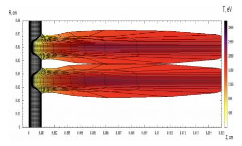
Figure 15. Plasma expansion on target front side at t = 0.18 ns showing the collision of the two plasma plumes. Here the target is  $10 \mu m$  Al irradiated by the laser with 50 J energy.
