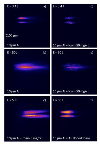
**Figure 4.** X-ray streak-camera images on target front side. Time goes from left to right with time window 2 ns.
