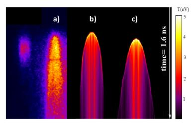
Figure 7. (a) Experimental results for  $10 \,\mu m$  Al target (from Figure (c)). (b) Temperature of the target rear side versus space and time from 2D simulations and a  $10 \,\mu m$  Al target. (c) The same for a target of  $10 \,\mu m$  Al + 50  $\,\mu m$  foam. In both cases the focal spot FWHM was  $70 \,\mu m$ , the time profile of the laser pulse was Gaussian, and the peak intensity was  $1.25 \times 10^{15}$  W/cm<sup>2</sup>.
