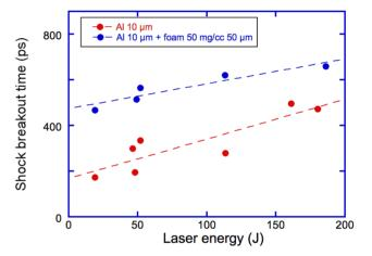
**Figure 5.** Shock breakout time versus laser energy for simple Al 10- $\mu$ m targets and for foam-layered Al targets (foam density 50 mg/cm<sup>3</sup>).
