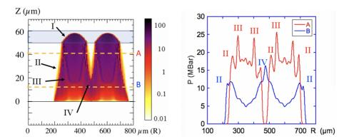
Figure 12. Time t = 0.4 ns: (left) hydro-simulations (as in Figure 11 but rotated by 90°); (right) pressure profiles at z = 18 and 47  $\mu$ m (dashed lines A and B in the figure on the left). Here (I) is the forward shock travelling in Al, (II) is the reverse shock travelling back in the foam, (III) is the forward shock, still expanding radially in the foam, and (IV) is the region where the two radially expanding shocks have collided.
