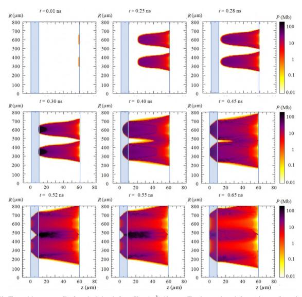
Figure 11. The spatial pressure profiles from simulations in foam (50 mg/cm<sup>3</sup>)–Al targets. The plots are shown in Lagrangian coordinates, i.e., R and z correspond to the initial position of each cell in the simulation mesh. In the images, the blue line and the blue rectangle show the position of the target (foam) surface and the position of the 10  $\mu$ m Al foil, respectively.
