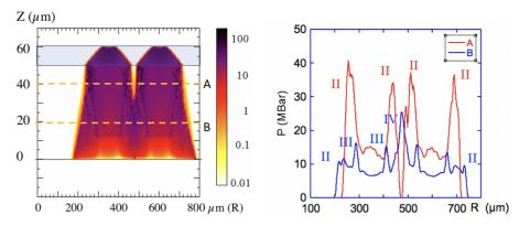
**Figure 13.** Time t = 0.45 ns: (left) hydro-simulations (as in Figure 11 but rotated by 90°); (right) pressure profiles at z = 18 and 41  $\mu$ m (dashed lines A and B on the left). Here (I) to (IV) are the same as in Figure 12. Note: in position A, the radial forward shocks (II) and the reverse shocks (III) have practically merged.
