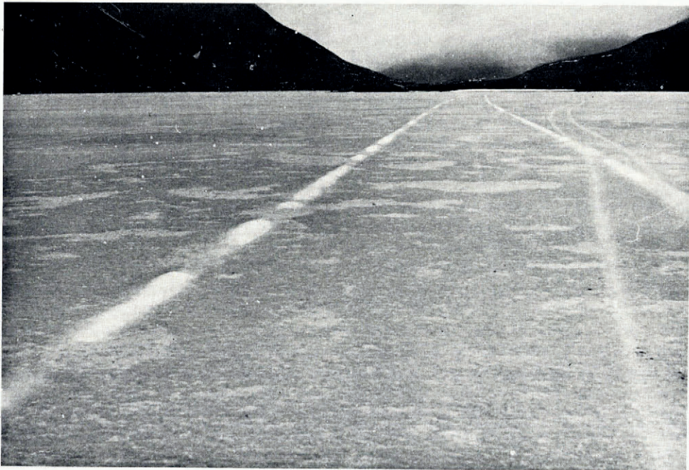
Fig. 3. The surface of Peters Lake showing patches of c-axis-vertical ice in c-axis-horizontal ice. Note the track of a taxiing DC-3 airplane; the wheels dug grooves about 20 cm. deep in canded, c-axis-horizontal ice but they made no impression on the c-axis-vertical ice
