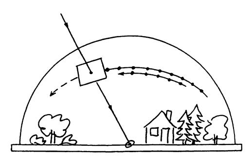
FIGURE 1. The plastic sphere for measuring the path of the Sun above the horizon. (Germany).
