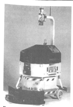
**Figure 1.** The Mobile Automated Characterization System can detect alpha and beta contamination on the floors. Department of Energy photo.
