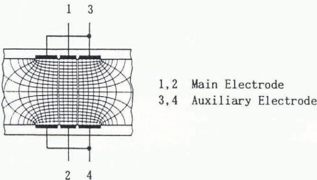
Fig. 1. Application of "auxiliary electrodes". The electrodes work to keep the potential gradient or the current density uniform between the main electrodes.
