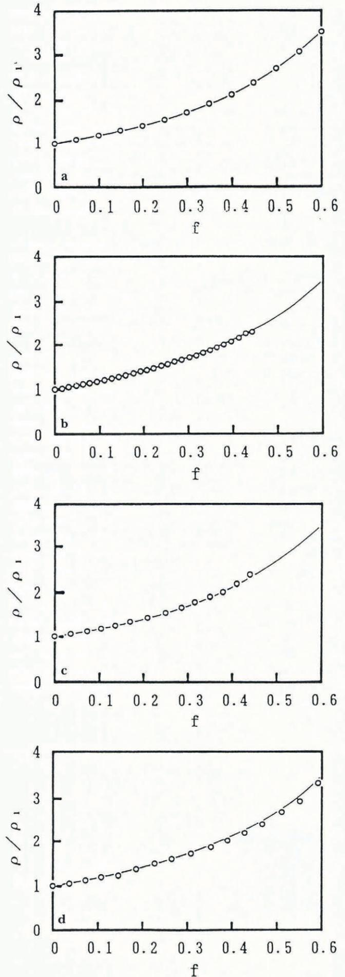
Fig. 4. Relative resistivity,  $\rho/\rho_1$ , vs volume fraction,  $f$ . The curve is authors' relation. a, ABS resin bead; b, rubber ball; c, granular snow; d, ice cube.
