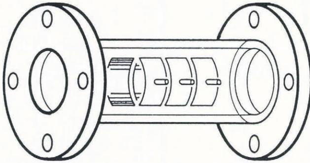
Fig. 6. An electrode-duct-section for pipeline system. Electrode pairs are fitted opposite each other in the duct.
