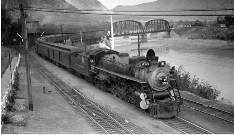
Figure 5: The railroad tracks down river from Glenwood Springs, c. 1930. Credit: D&RGW train, engine number 1703, engine type 4-8-4, c. 1930, Western History Collection, OP-10398 (Denver Public Library, Denver, CO).
