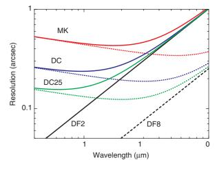
**Figure 4** Resolution attainable with a 2-m telescopes (solid lines) and an 8-m telescope (dotted lines) at both Dome C and Mauna Kea, as a function of wavelength. The resolution is calculated by adding, in quadrature, the seeing to the diffraction limit. Curves are shown for Mauna Kea (red), median seeing conditions at Dome C (blue) and for the best 25% conditions at Dome C (green). Also shown in black, for comparison, is the diffraction-limited performance for a 2-m and an 8-m telescopes.
