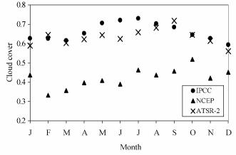
Fig. 4. Mean monthly cloud cover for a transect at  $65.7^{\circ}N$ determined from the IPCC meteorological observations, NCEP re-analysis data for 1997 and ATSR-2 stereo-matching, with a maximum in late summer and a minimum in winter. The NCEP values are considerably lower due to the exceptionally low cover reported for the centre of the ice sheet.
