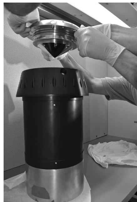
**Fig. 20.** Mating the mirror assembly to the front of the VALKYRIE beam dump.
