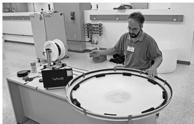
Fig. 4. Preparing 1050 m of fiber for the initial high-power transmission test.
