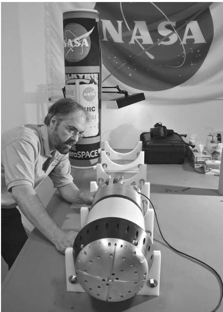
**Fig. 22.** Assembled VALKYRIE prototype beam dump and melt head.
