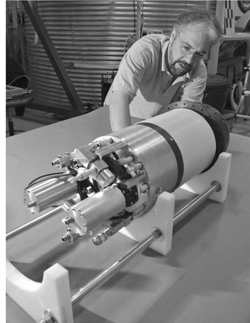
**Fig. 23.** Hot-water jet pumps, filters and valve assemblies on the back of the beam dump.
