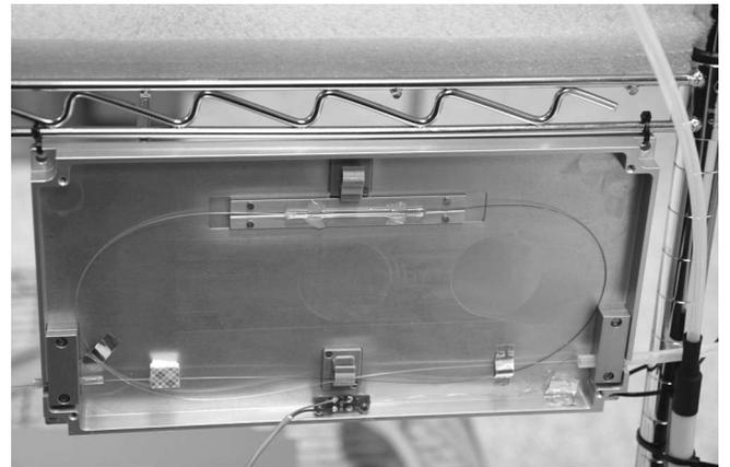
Fig. 7. Fiber splice for initial high-power tests.
