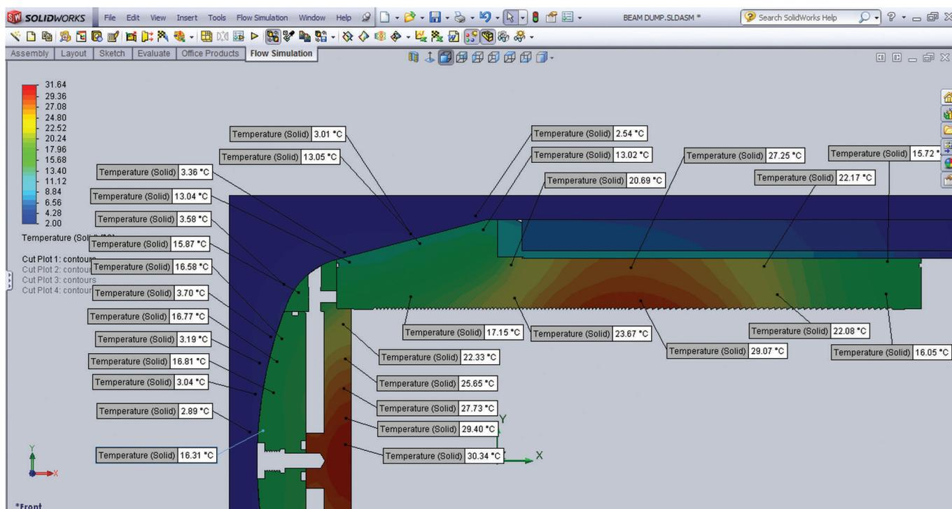
Fig. 26. Steady-state beam dump temperatures at 5 kW and failed water jet pumps.
