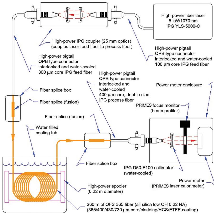
**Fig. 10.** Set-up diagram for high-power tests of the VALKYRIE fiber spooler.
