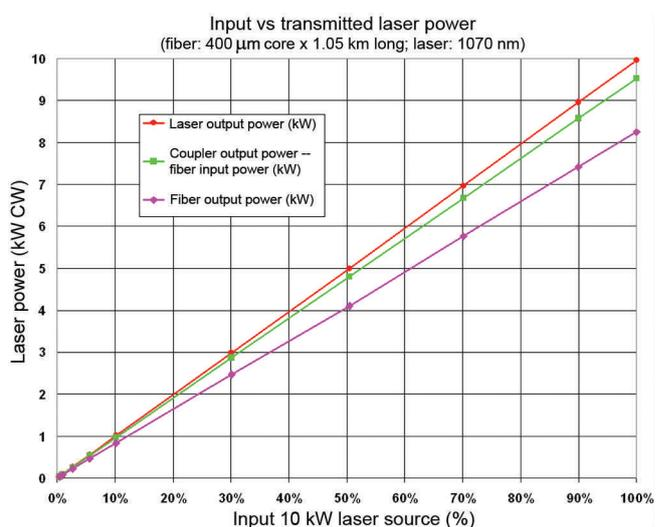
**Fig. 8.** Transmission power results from first high-power test.
