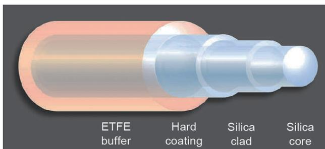
**Fig. 11.** Schematic of the optical waveguide layers used for the spooler tests.
