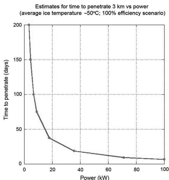
Fig. 3. Mission duration as a function of input power for a 0.25 m diameter cryobot.
