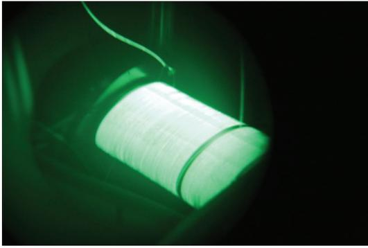
**Fig. 13.** Infrared image of the VALKYRIE fiber spooler at 5 kW power input.
