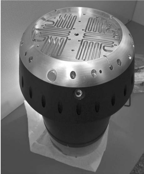
**Fig. 21.** Cooling channels on the back side of the beam dump for mirror cooling.
