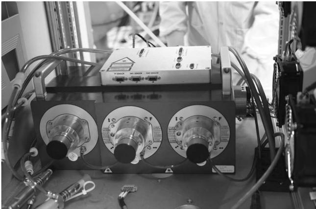
Fig. 6. High-power laser fiber switch.
