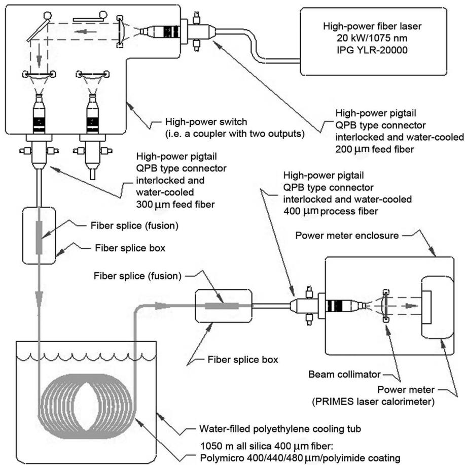
Fig. 5. Schematic of initial high-power transmission test.
