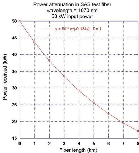
**Fig. 16.** Theoretical power delivered to VALKYRIE as a function of spooler length for 50 kW input power.
