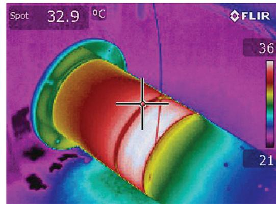
**Fig. 14.** Thermal camera image showing steady-state temperature distribution on the fiber spooler mock-up at 5 kW input power.
