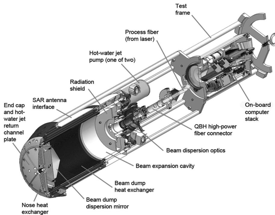
**Fig. 18.** Solid model section of the initial test prototype for VALKYRIE.
