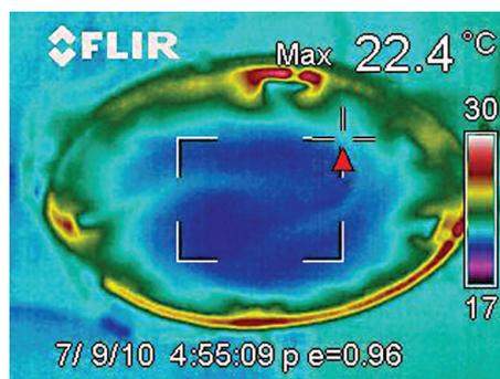
**Fig. 9.** Thermal camera image showing temperature of the 1050 m fiber spool at steady-state full power (10 kW).
