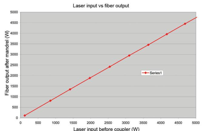
**Fig. 15.** Power output from the spooler as a function of input power.
