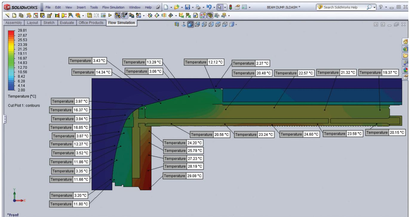
Fig. 27. Steady-state beam dump temperatures at 5 kW with internal recycling of water.
