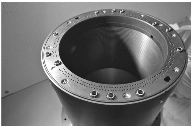
**Fig. 19.** Rear view of the VALKYRIE beam dump heat exchanger.
