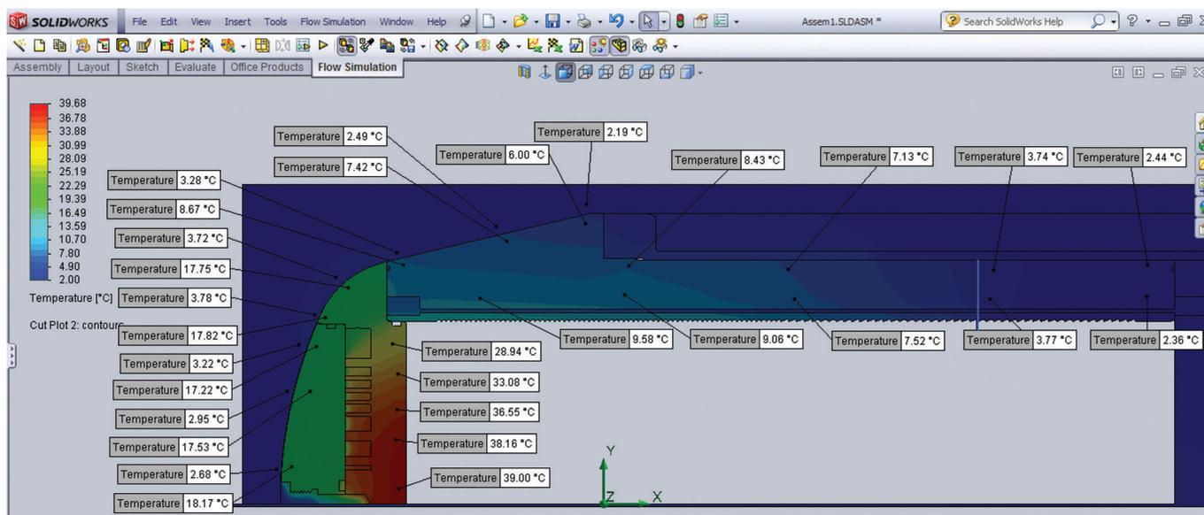
Fig. 25. Steady-state beam dump temperatures at 5 kW with water jets operating.
