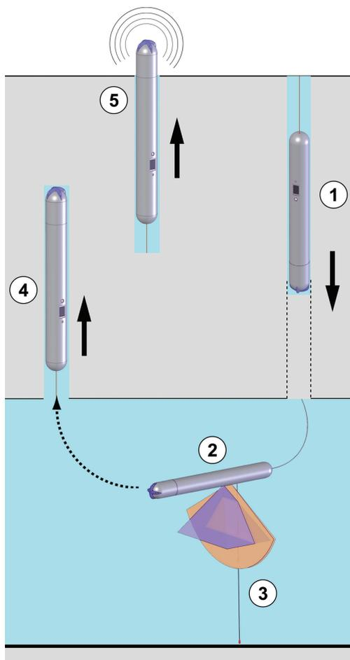
Fig. 28. Envisioned subglacial lake sample return mission: (1) descent through the ice cap; (2) vehicle pitch-up maneuver and conversion to AUV; (3) bottom sample acquisition and bathymetric mapping; (4) vehicle pitch-up maneuver with center of gravity shifting and buoyancy increase; and (5) return to surface.
