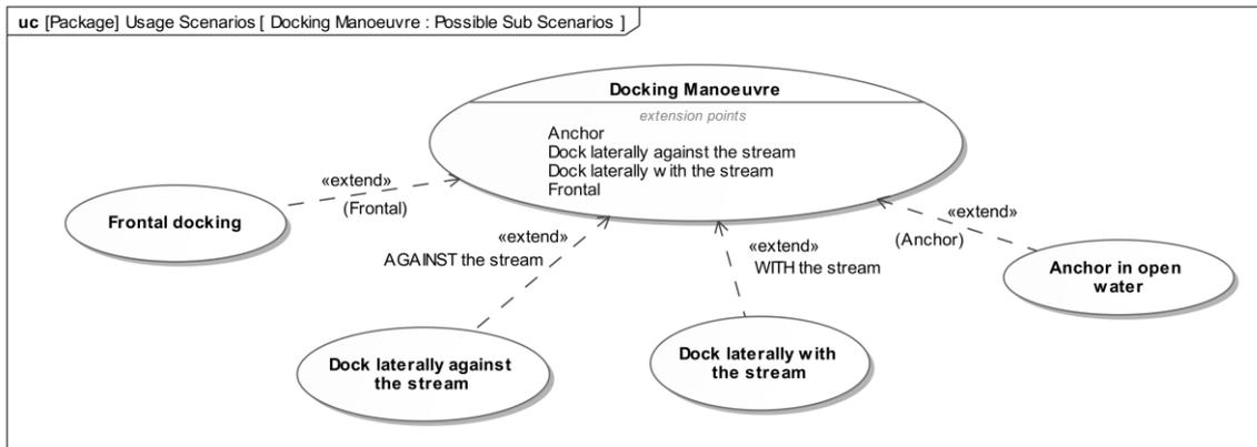
Figure 5. Possible sub scenarios on the usage phase of the base scenario “Docking Manoeuvre”
