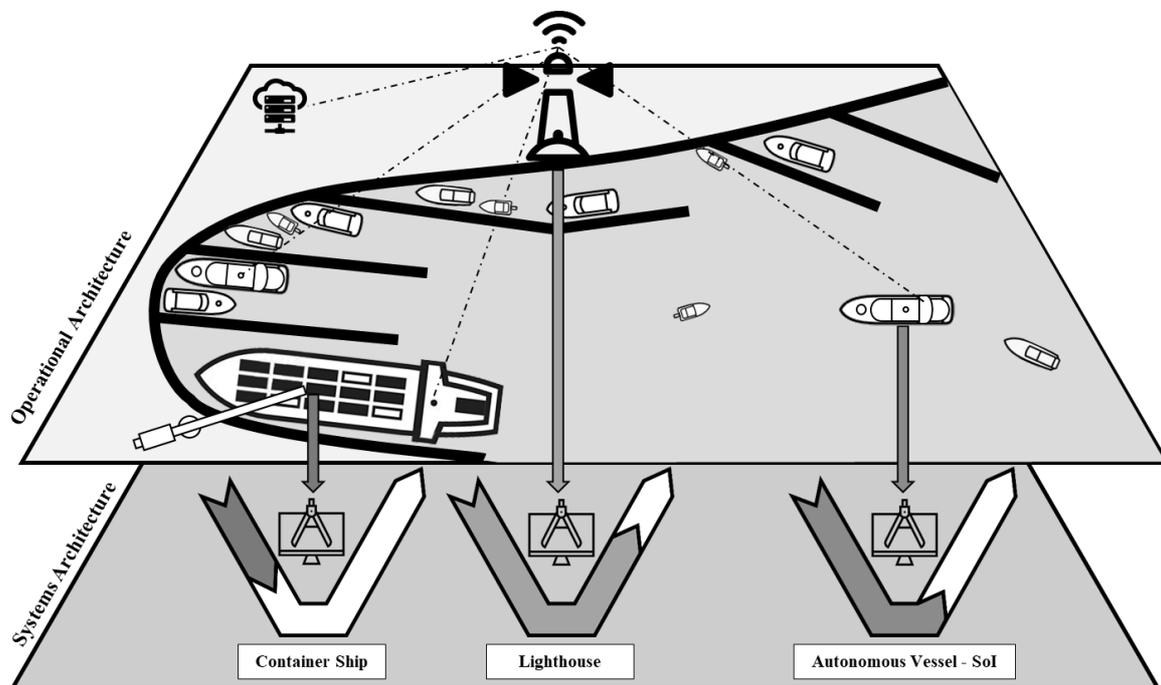
**Figure 1. Depiction of the differentiation between the SoI architecture and the operational architecture of a SoS on the example of an autonomous docking scenario**
