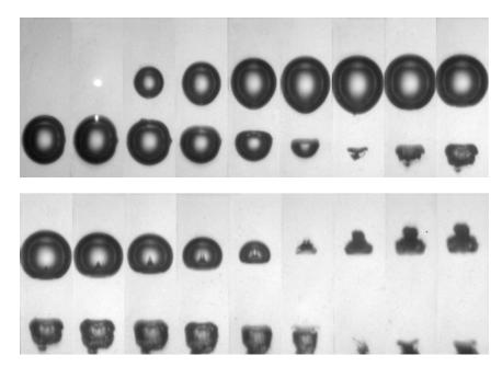
FIGURE 6. Dynamics of an anti-phase bubble pair ( $\tau = 1$ ) with bubbles of approximately equal size ( $\rho = 1$ ). The bubble distance d at initiation is d = 2.5 mm;  $R_{max} = 1.0$  mm,  $\gamma = 1.25$ . The frame interval is 20 µs.
