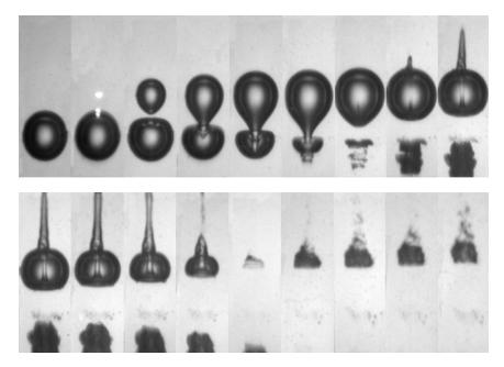
FIGURE 8. Dynamics of an anti-phase bubble pair ( $\tau = 1$ ) with bubbles of approximately equal size ( $\rho = 1$ ). The bubble distance d at initiation is d = 1.5 mm;  $R_{max} = 1.0$  mm,  $\gamma = 0.75$ . The frame interval is 20 µs.
