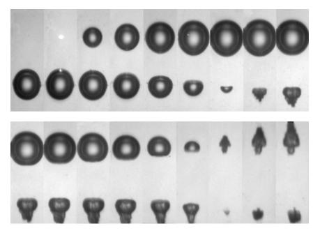
FIGURE 5. Dynamics of an anti-phase bubble pair ( $\tau = 1$ ) with bubbles of approximately equal size ( $\rho = 1$ ). The bubble distance d at initiation is d = 3.0 mm;  $R_{max} = 1.0$  mm,  $\gamma = 1.5$ . The frame interval is 20 µs.
