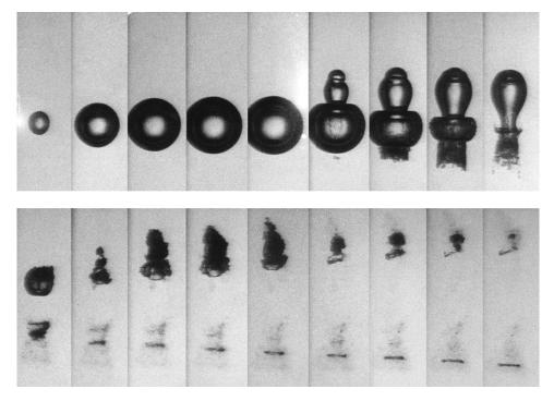
FIGURE 9. Dynamics of an anti-phase bubble pair ( $\tau = 1$ ) with bubbles of approximately equal size ( $\rho = 1$ ). The bubble distance d at initiation is d = 3 mm;  $R_{max} = 2.1$  mm,  $\gamma = 0.715$ . The frame interval is 50 µs. Taken from Lauterborn & Hentschel (1985).
