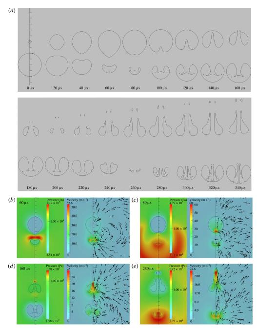
FIGURE 14. Dynamics of an anti-phase bubble pair. Simulation parameters are  $R_{max1} = 1 \text{ mm}$ ,  $R_{max2} = 1.04 \text{ mm}$  and  $\gamma = 1.0$ . (a) Bubble shapes; and (b-e) selected frames from the simulation with pressure and velocity fields. To be compared with experimental results from figure 7 with  $R_{max1} \approx 1 \text{ mm}$  and  $\gamma \approx 1.0$ . The numerical peak jet velocities of bubble 1 and bubble 2 are both about 30 m s<sup>-1</sup>.
