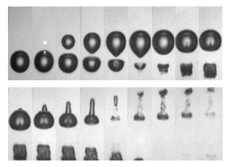
FIGURE 7. Dynamics of an anti-phase bubble pair ( $\tau = 1$ ) with bubbles of approximately equal size ( $\rho = 1$ ). The bubble distance d at initiation is d = 2 mm;  $R_{max} = 1.0$  mm,  $\gamma = 1.0$ . The frame interval is 20 µs.
