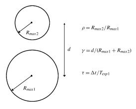
FIGURE 1. Illustration of parameters governing laser-induced bubble pair dynamics. Bubble 1 is produced first, bubble 2 after a delay time  $\Delta t$ . Time  $T_{exp1}$  is the expansion time of bubble 1 after which it reaches its maximum radius  $R_{max1}$ .
