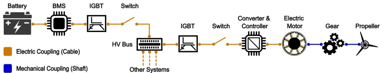
Figure 1. Simplified topology of an electric aircraft powertrain (according to Stückl (2016))
