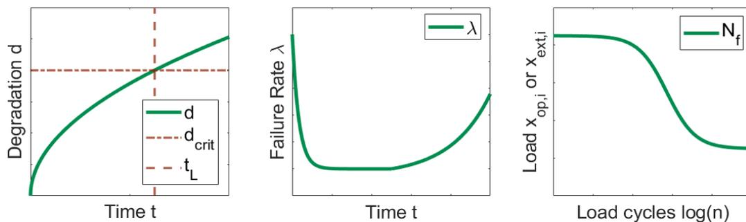
Figure 3. Degradation (left), failure rate (middle) and load cycles (right) as basic model approaches for lifetime prognosis
