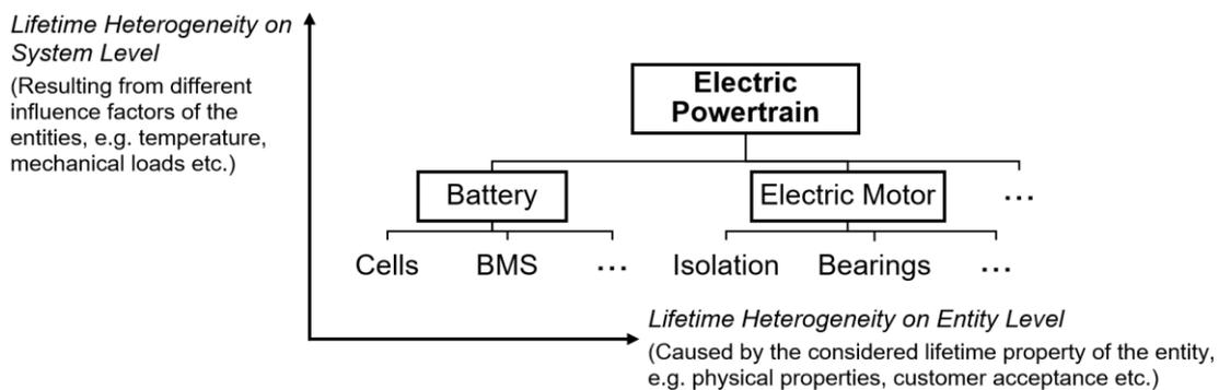
Figure 2. Concept of lifetime heterogeneity on system and entity level
