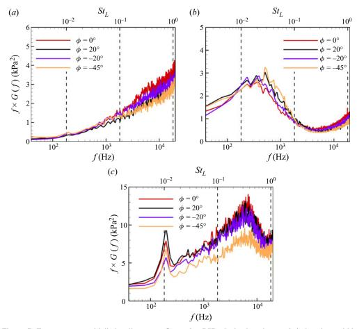
Figure 7. Frequency-premultiplied wall pressure fluctuation PSD obtained at characteristic locations within the SBLI unit over different azimuthal locations: (a) separation bubble ( $x \approx -3\delta$ ), (b) intermittent region ( $x \approx -9.5\delta$ ) and (c) reattachment location ( $x \approx +2.1\delta$ ).
