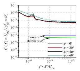
Figure 5. Comparison of wall pressure fluctuation PSD obtained beneath the incoming boundary layer at different azimuthal locations. Comparisons with previous measurements from Beresh *et al.* (2011) and the empirical predictions of Lowson (1968) are also presented.
