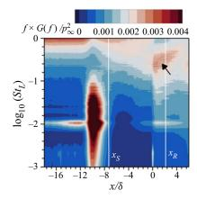
Figure 8. Streamwise evolution of frequency-premultiplied pressure fluctuation PSD obtained at  $\phi = 0^{\circ}$ . The abrupt occurrence of the PSD elevation at  $St_L \approx 0.2$ –0.4 is indicated by an arrow.
