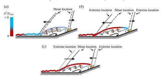
Figure 15. Illustration of the mechanisms that drive the different phases of separation bubble motion: (a) gradual expansion, (b) rapid expansion and (c) relaxation to mean separation size.
