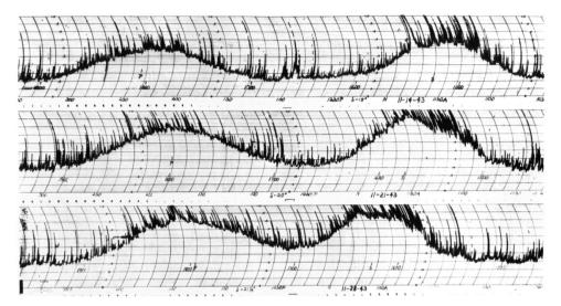
Figure 1.13 Reproduction of Reber's 160 MHz chart recordings from three separate days in late 1943. Each scan is at a different declination. The two bumps indicate the plane of the Milky Way on the left and the Sun on the right. The multiple sharp spikes show ignition noise from passing automobiles. Credit: NRAO/AUI Archives, Papers of G. Reber.
