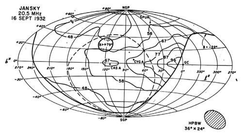
Figure 1.9 Contour map plotted in galactic coordinates showing the distribution of radio intensity over the sky, constructed by Woodruff T. Sullivan III from Jansky's 16 September 1932 data. Courtesy of W. T. Sullivan III.
