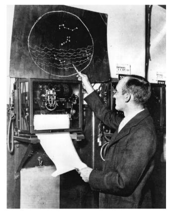
Figure 1.6 Karl Jansky in 1933 at the chart recorder output of his 21 MHz radiometer. Credit: Nokia Corporation and AT&T Archives.
