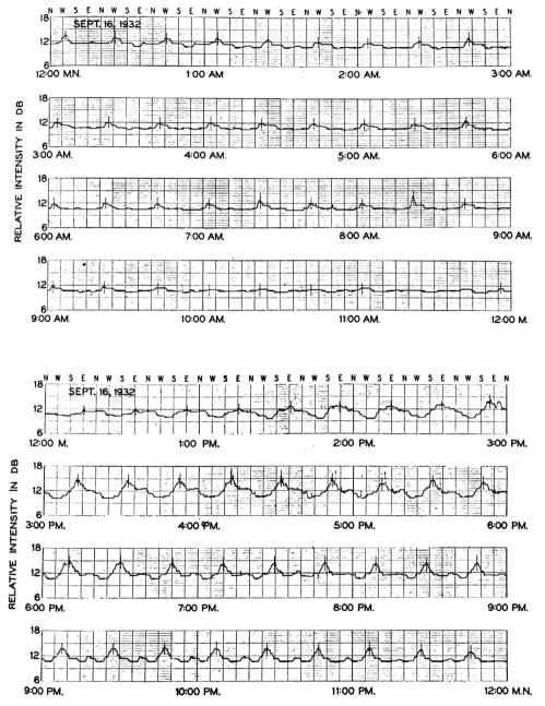
Figure 1.8 Reproduction of Jansky's 16 September 1932 chart recorder output showing the radio emission from the Milky Way in a 12 hour period as his antenna beam swept across the Galaxy three times an hour. The different response profiles reflect the varying angle of Jansky's fan beam alignment with the plane of the Milky Way. The lettering at the top of each plot indicates the direction of the antenna beam at that time. Credit: NRAO/AUI Archives, Papers of W.T. Sullivan III.
