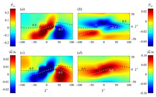
Figure 15. Colour maps of the components of the turbulence production (a)  $\tilde{\mathcal{P}}_{xx}$  and (b)  $\tilde{\mathcal{P}}_{xz}$ , and corresponding components of the velocity gradient (c)  $\partial \tilde{u}/\partial x$  and (d)  $\partial \tilde{u}/\partial z$  calculated over the VISA events, overlaid with the isolines  $\tilde{u}^+ = \pm 0.5$ .
