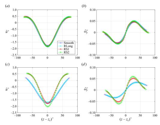
Figure 4. Conditionally averaged (a,c) streamwise velocity fluctuations and (b,d) wall-normal vorticity profiles, calculated across the LSS. Data are collected at (a,b)  $Re_{\theta} = 2200$  and  $y^+ = 35$ , (c,d)  $Re_{\theta} = 2900$  and  $y^+ = 50$ .
