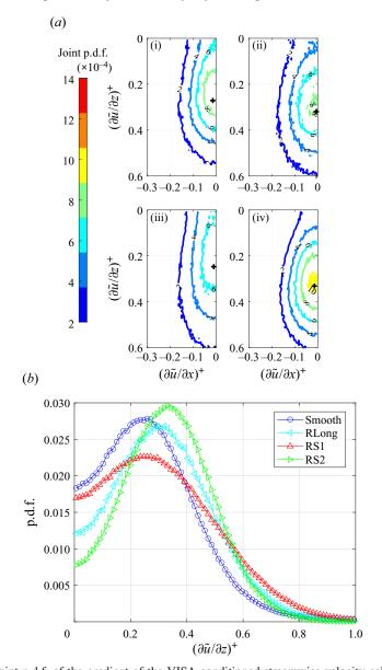
Figure 13. (a) Joint p.d.f. of the gradient of the VISA conditioned streamwise velocity calculated along the streamwise  $((\partial \tilde{u}/\partial x)^+)$  and cross-stream  $((\partial \tilde{u}/\partial z)^+)$  directions at the centre of each VISA event for the (i) Smooth, (ii) RLong, (iii) RS1 and (iv) RS2 cases. (b) Marginal p.d.f. of  $(\partial \tilde{u}/\partial z)^+$ . Data are collected at  $Re_\theta = 2900$  and  $y^+ = 50$ .
