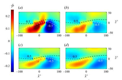
Figure 14. Colour map of the VISA conditionally averaged production  $(\tilde{P})$ , overlaid with the isolines  $\tilde{u}^+ = \pm 0.5$ , for the (a) Smooth, (b) RLong, (c) RS1 and (d) RS2 cases. Data are collected at  $Re_{\theta} = 2900$  and  $y^+ = 50$ .
