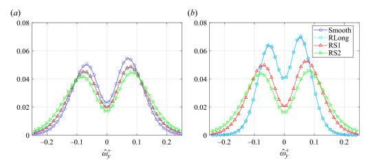
Figure 6. Probability density functions of the wall-normal vorticity  $\hat{\omega}_y$  calculated at the streaks' edges. Data are collected at (a)  $Re_{\theta} = 2200$  and  $y^+ = 35$ , (b)  $Re_{\theta} = 2900$  and  $y^+ = 50$ .
