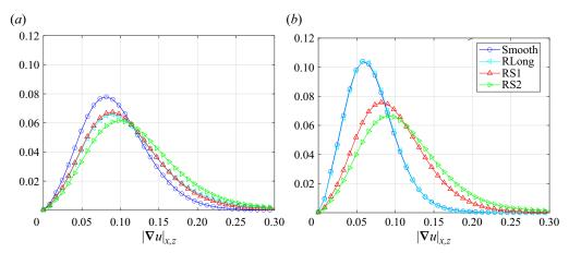
Figure 5. Probability density functions of the modulus of the velocity gradient ( $|\nabla \hat{u}|_{x,z}$ ) projected on the x-z plane calculated at the streaks' edges, for (a)  $Re_{\theta} = 2200$  and  $y^+ = 35$ , (b)  $Re_{\theta} = 2900$  and  $y^+ = 50$ .
