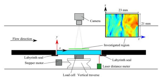
Figure 1. Schematic representation of the test section with detail of the removable plate. The track of the laser sheet, indicated in green, is not to scale. The inset reports a representative snapshot with the indication of the streamwise and spanwise extents of the measurement region.
