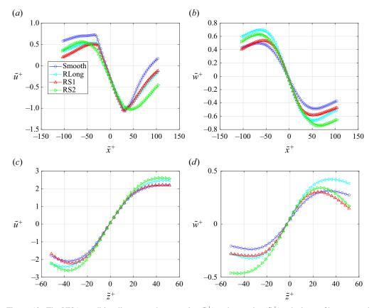
Figure 12. The VISA conditionally averaged streamwise  $(\tilde{u}^+)$  and spanwise  $(\tilde{w}^+)$  velocity profiles extracted at (a,b)  $z^+=0$  and (c,d)  $x^+=0$  for VISA events characterized by  $\partial u/\partial x<0$  and  $\partial u/\partial z>0$ , with overlaid streamlines. Data are collected at  $Re_\theta=2900$  and  $y^+=50$ .
