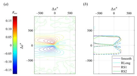
Figure 9. (a) Contour plot of the normalized two-point correlations  $R_{uw}$  calculated for the Smooth case. (b) Comparison between the four investigated cases for one generic contour line,  $R_{uw} = \pm 0.04$  (solid/dashed line, respectively). Data are collected at  $Re_{\theta} = 2900$  and  $y^{+} = 50$ .
