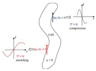
Figure 16. Schematic representation of the relation between the velocity gradient and the values of the turbulence production.
