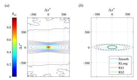
Figure 7. (a) Contour plot of the normalized two-point correlations  $R_{uu}$  calculated for the Smooth case. (b) Comparison between the four investigated cases for two generic contour lines:  $R_{uu} = 0.5$  (solid line)  $R_{uu} = 0.2$  (dashed line). Data are collected at  $Re_{\theta} = 2900$  and  $y^+ = 50$ .
