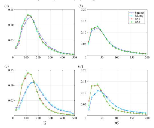
Figure 3. Probability density function of the streaks' (a,c) spacing and (b,d) width. Data are collected at (a,b)  $Re_{\theta} = 2200$  and  $y^{+} = 35$ , (c,d)  $Re_{\theta} = 2900$  and  $y^{+} = 50$ .
