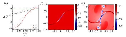
Figure 3. Vorticity generation with We = 12, At = 0, Re = 10114. (a) Velocity jump measured across the interface, as a function of interface location within the vortex core. Symbols: DNS, line: (3.3). The perturbation vorticity from the DNS is shown for time  $t_n = 1$  in (b) and for  $t_n = 15$  in (c). The instability is well developed by  $t_n = 15$ . All lengths are scaled by  $r_c$ .
