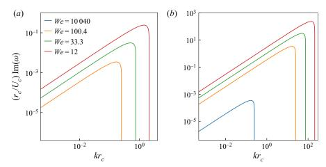
Figure 2. Non-dimensional growth rate of perturbations ( $r_c \text{Im}(\omega)/U_c$ ) on the interface vs the wavenumber  $kr_c$ ; (a)  $t_n=1$  and (b)  $t_n=5$ . Here,  $r_c=0.1$  and At=0. As We decreases, the growth rate increases, showing the destabilising effect of surface tension.
