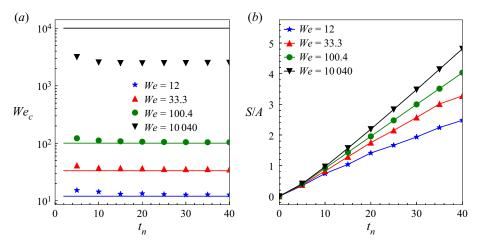
Figure 6. (a) Weber number estimated by the energy balance (symbols) compared against the actual Weber number (lines). (b) Increase in interface length (scaled by total area) with time.
