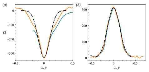
Figure 11. Comparison of the vorticity profile for vortices 1,2 shown in figure 10(b) with the best fitting Lamb-Oseen vortex (Gaussian). Vorticity variation along x and y for (a) vortex 1 and (b) vortex 2. The black dashed lines represent the fit to a Lamb-Oseen vortex  $\Omega \equiv \Omega_0 \exp(-q)$ , where  $\Omega_0$  is the maximum vorticity and  $q = (x^2 + y^2)/r_c^2$ . The origin in each case is at the vortex core.
