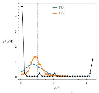
Figure 9. Value of P(a/A) versus a/A for two runs TR2,  $We = 5 \times 10^5$  and TR4,  $We = 5 \times 10^3$  time averaged from  $14.1\tau_e$  to  $14.6\tau_e$ . Black dashed line corresponds to a/A = 1. The black solid line with circles represents the p.d.f. for a circular patch of minority fluid of the same volume fraction (=0.225) as that of the minority fluid in the simulations. As the We increases, most boxes have the same volume fraction as that of the total domain.
