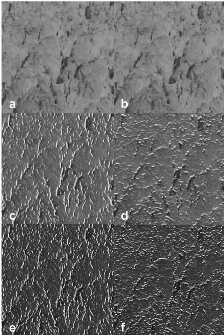
**Fig. 4.** (a) Original image, (b) intensity image and (c) 0° edge-enhanced, (d) 90° edge-enhanced, (e) 0° edge + high-frequency enhanced and (f) 90° edge + high-frequency enhanced images of a heavily crevassed portion of an image of Rink Isbræ.
