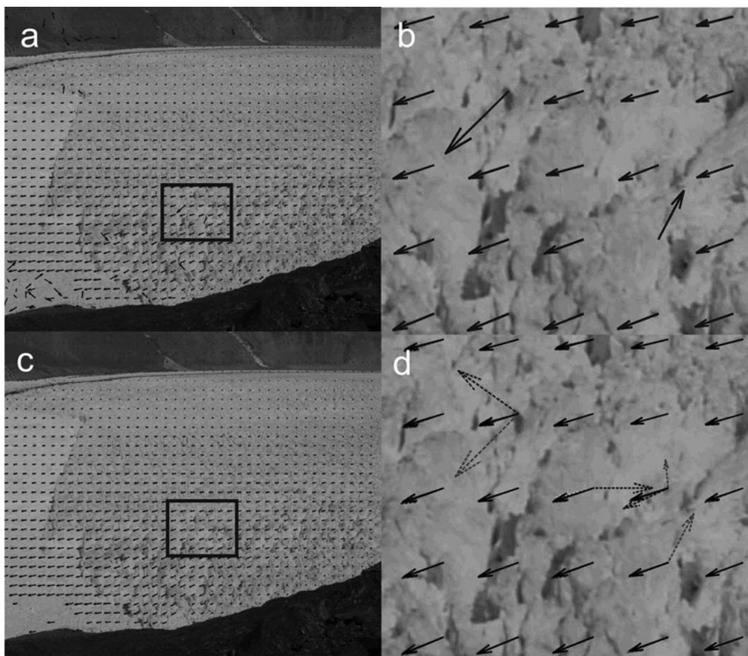
**Fig. 5.** Illustration of 30 × 30 reference chip red-band displacement results from conventional matching (a, b) and from MIMC (c, d). Dashed arrows indicate outliers removed by the voting cell approach. Dashed arrows in (d) indicate cases where conventional matching fails.
