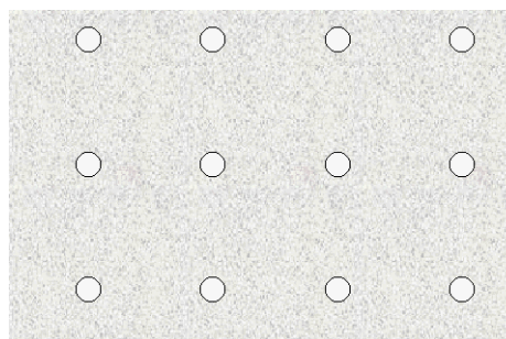
Figure 2. Schematic of the pattern used for the selective area coverage of the sapphire substrates. Textured area represents the \text{SiO}_2 layer while the clear circles show the exposed sapphire substrate.
