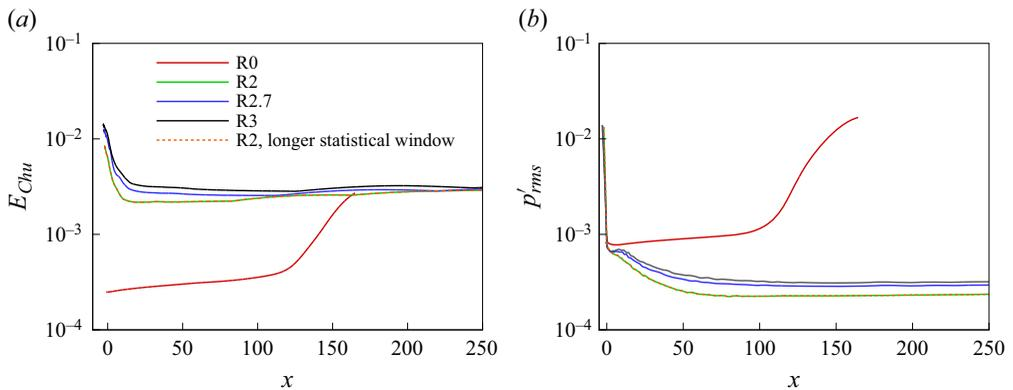
Figure 7. (a) Chu's energy and (b) the r.m.s. of wall pressure fluctuations for 2-D cases. Statistics are performed in an interval  $t^* = 1$  ms (at least 3.5 flow-through time units). The 'longer statistical window' corresponds to another statistical interval of 2 ms.
