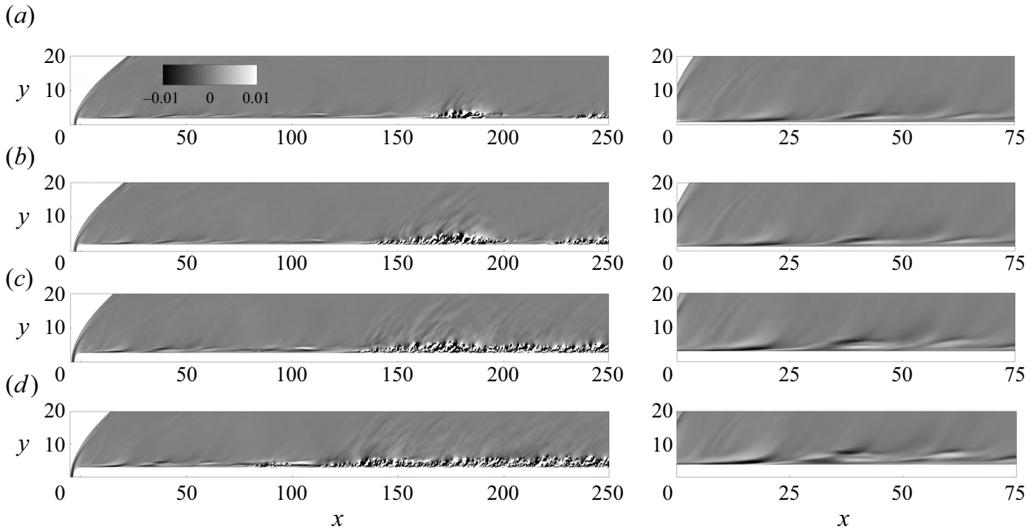
Figure 18. Instantaneous spanwise velocity  $w$  on the symmetry plane  $z = L_z/2$  at  $t = 806$  for cases (a) R1.8, (b) R2, (c) R2.7 and (d) R3. The characterisation of the leading-edge streak is highlighted in the right-hand column. The contour level ranges from  $-0.01$  to  $0.01$ .
