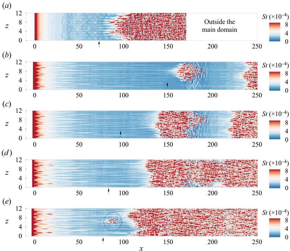
Figure 13. Contour of instantaneous Stanton number at  $t = 806$  for cases (a) R0, (b) R1.8, (c) R2, (d) R2.7 and (e) R3. The circle in (e) marks the early turbulent spots. Arrows represent the transition onset locations.
