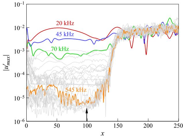
Figure 25. Development of the local maximum of the streamwise velocity fluctuation  $|u'_{max}|$  for the first leading SPOD  $x$ - $y$  mode for case R2C. Different frequencies are displayed with an interval of 25 kHz starting from 20 kHz, among which four frequencies are highlighted (20, 45, 70, 545 kHz). Envelopes of the signal are taken from the original SPOD  $|u'_{max}|$  to highlight the overall evolution. The arrow represents the transition onset location.
