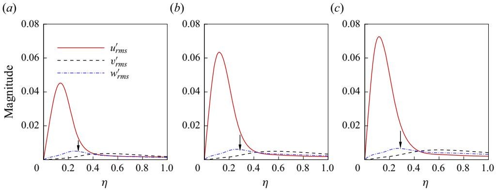
Figure 15. Wall-normal profiles of spanwise-averaged r.m.s. of velocity fluctuations  $u', v', w'$  at the laminar-flow position  $x = 20$  for cases (a) R2, (b) R2.7 and (c) R3. Arrows represent the locations of local laminar-boundary-layer thickness.
