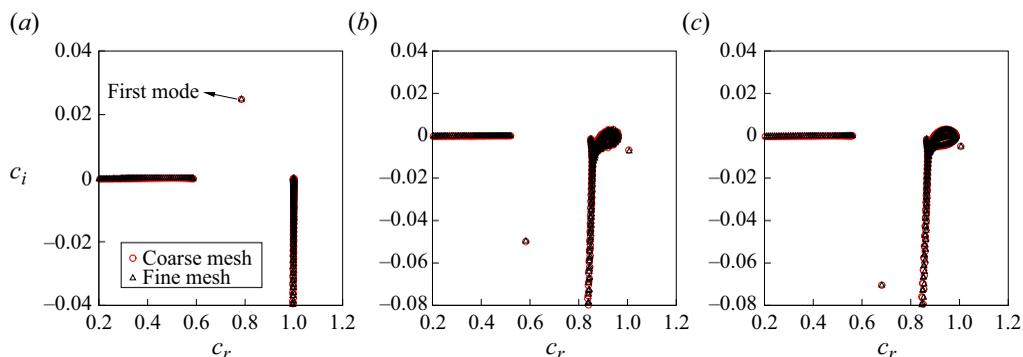
Figure 9. Eigenspectrum of the complex phase velocity  $c = \omega/\alpha$  with  $\omega = 0.9$  and  $\beta = 2.75$  for (a) case R0 at  $x = 50$ , (b) case R2 at  $x = 50$ , and (c) case R2 at  $x = 150$ .
