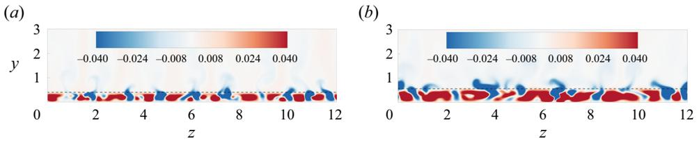
Figure 12. Contour of the streamwise velocity perturbation  $u_{perturb}$  compared to the laminar flow of case R3 at  $t = 806$  for (a)  $x = 40$  and (b)  $x = 80$ . Dashed lines mark the position of the 2-D laminar boundary layer edge.
