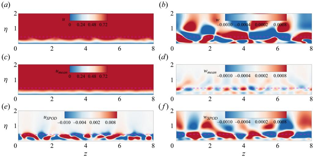
Figure 27. (a,b) Instantaneous, (c,d) time-averaged and (e,f) SPOD-modal quantities of the first leading SPOD  $z$ - $y$  mode with  $f^* = 20$  kHz for case R2C, including (a,c,e) streamwise velocity and (b,d,f) spanwise velocity. The slice is extracted in the pre-transitional region  $x = 50$ . The dashed line represents the location of the 2-D laminar-boundary-layer thickness.
