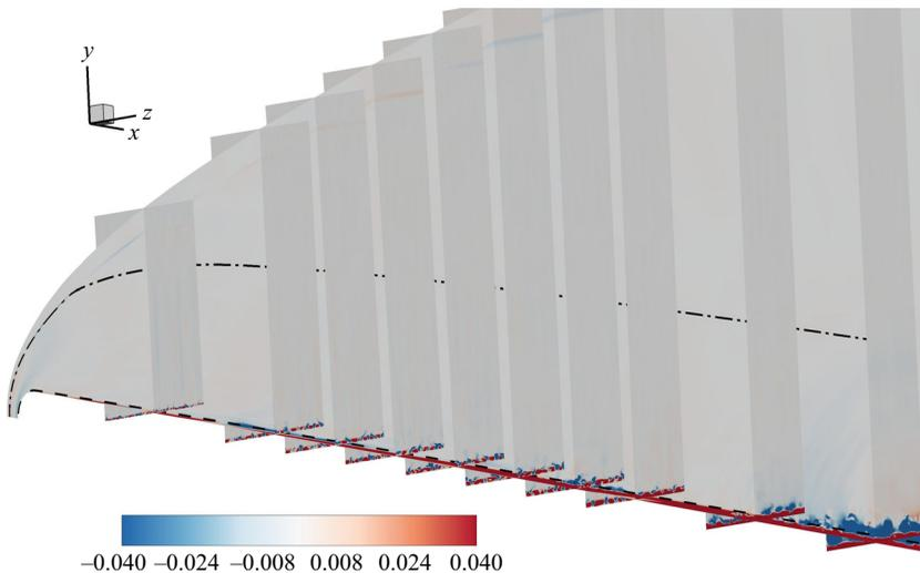
Figure 31. Contour of the streamwise velocity perturbation  $u_{perturb}$  compared to the laminar flow for case R3 at  $t = 806$ . Dashed and dash-dotted lines mark the boundary-layer edge and the entropy-layer edge, respectively. Transverse slices are extracted and shown with  $x$ -coordinates 20, 40, 50, 60, 70, 80, 90, 120 and 140, successively.
