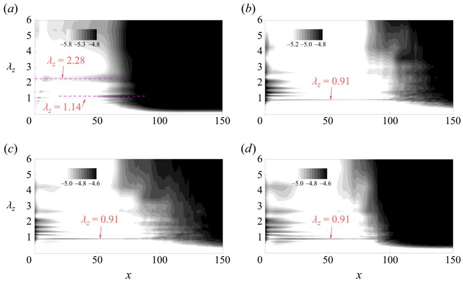
Figure 19. Common logarithm of modulus of spanwise Fourier transforms of Stanton number  $\log_{10}(|\tilde{S}r|)$  versus the streamwise coordinate  $x$  and the spanwise wavelength  $\lambda_z$  for cases (a) R0, (b) R2, (c) R2.7 and (d) R3. The ensemble average of the result is taken during  $t_2 - t_1 = 800$ .
