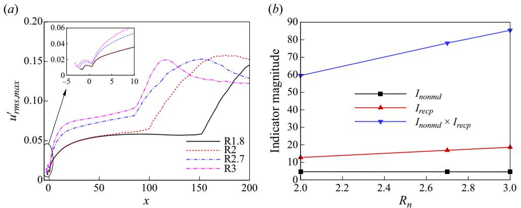
Figure 17. (a) Local maximum of spanwise-averaged  $u'_{rms}$  versus  $x$ . (b) Indicators of the significance of receptivity or non-modal growth subject to the nose bluntness effect. The leading-edge reference location is  $x_{LE} = 0$ .
