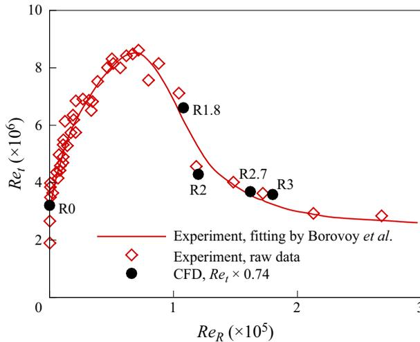
Figure 3. Plot of transition onset Reynolds number versus nose-tip radius Reynolds number. The original experimental Reynolds number based on the leading-edge thickness  $b = 2R_n$  is transformed into the nose-tip-radius-based Reynolds number.
