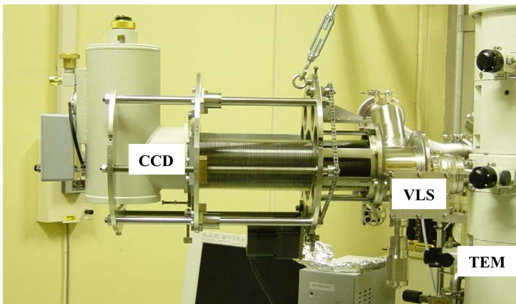
FIG.2 Photo of the spectrometer (3<sup>rd</sup> version) attached to a transmission electron microscope of JEM2000FX.
