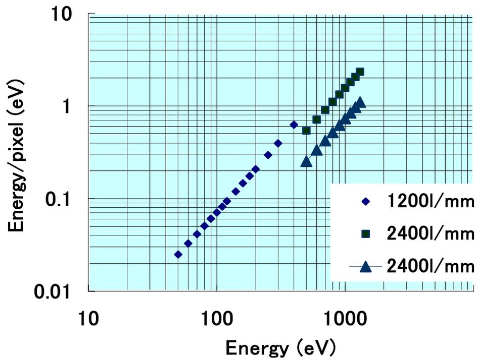
FIG.1 Energy dispersions (energy / CCD pixel) of the gratings of 1200 l/mm (◆), 2400 l/mm (■) already used and the newly designed grating of 2400 l/mm (▲).
