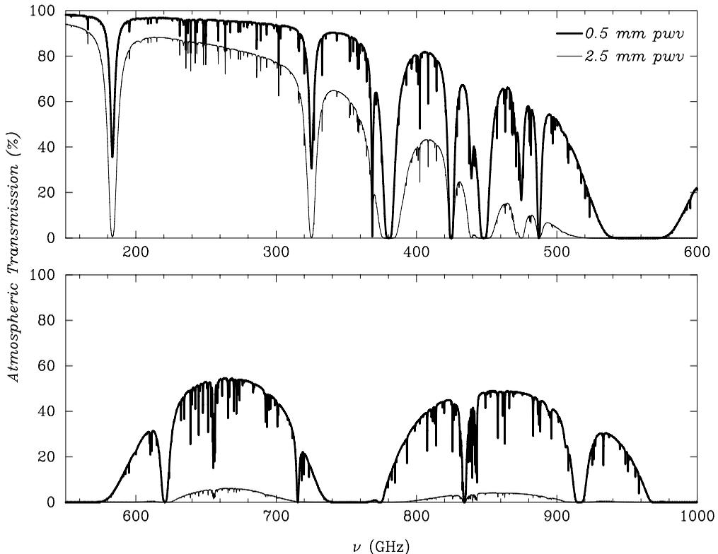
**Figure 2.** Zenith atmospheric transmission at Mauna Kea for column densities of 0.5 and 2.5 mm  $\text{H}_2\text{O}$  ( $\tau_{225\text{GHz}} \sim 0.04$  and  $0.13$  respectively). Data are from the Caltech Submillimeter Observatory Atmospheric Transmission Interactive Plotter (<http://www.submm.caltech.edu/cso/weather/atplot.shtml>).
