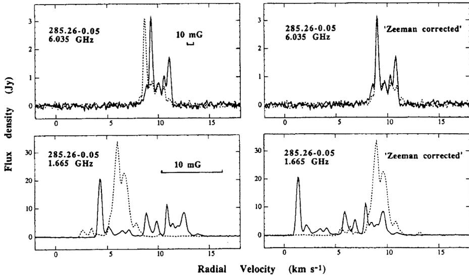
Figure 2. Observed spectra in LH panels show displacement of the 2 senses of circular polarization (LHCP broken line, RHCP continuous), attributable to the Zeeman effect. RH panels show the inferred velocities of emitted radiation when 'corrected' for Zeeman splitting.
