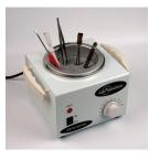
Heat guns and blow dryers are a fire hazard. Quickly and safely warm up all cryo-EM sample preparation tools using an inert medium. With the Cryo-Dryer there is no noise or unsafe air turbulence nearby. Warm up clipping stations, pucks, and anything else that can fit in the vessel. The system comes in a 110 V or 220 V configuration for use worldwide.
