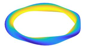
FIGURE 8. Three-dimensional plot of the classical stellarator boundary as described by (4.1)–(4.2). Colours indicate the magnetic field strength.
