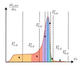
FIGURE 4. Sketch of pressure driven current density. Coloured area corresponds to the MRxMHD surface current. Black dashed lines represent volume interfaces.
