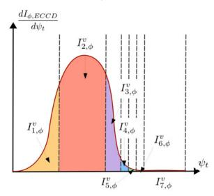
FIGURE 3. Sketch of externally driven current density (red curve). Coloured area corresponds to the MRxMHD volume current. Black dashed lines represent volume interfaces.
