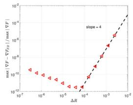
FIGURE 10. Normalized maximum absolute error between SPEC force gradient and a finite difference estimate in the case of a rotating ellipse. The dashed line has slope of four.
