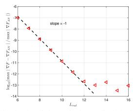
FIGURE 7. Semilogarithmic plot of the maximal normalized absolute error between the analytical force gradient,  $\nabla F_{AN}$ , and the force gradient obtained from SPEC,  $\nabla F$ , as a function of the radial resolution for the screw pinch case.
