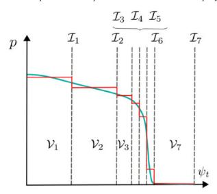
FIGURE 2. Sketch of a pressure profile as a function of the toroidal flux. Blue, continuous pressure profile obtained via experiment or analytical model; red, SPEC discretized pressure profile; black dashed lines, volume interfaces.
