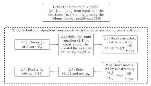
FIGURE 5. Flow of the algorithm used to constrain the net toroidal current profiles for a given toroidal flux profile and geometry.
