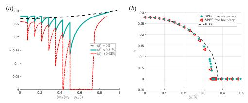
FIGURE 12. (a) Rotational transform profile at three different values of  $\langle \beta \rangle$ , for free-boundary calculation of a rotating ellipse with zero net toroidal current. (b) Rotational transform at the plasma edge as a function of  $\langle \beta \rangle$ . Comparison between free-, fixed-boundary and the HBS theory.
