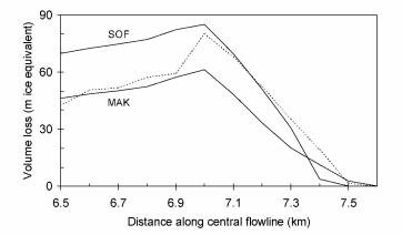
Fig. 7. Comparison between observed (dashed line) and modelled (solid lines) volume loss in the glacier front zone, 1952–2000. Results are shown for forcings with the SOF and MAK profiles.
