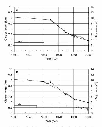
Fig. 5. Result of the dynamic calibration for SOF (a) and MAK (b) profiles. The observed glacier stands are marked by black dots. The lower solid line is the reconstructed mass-balance history.
