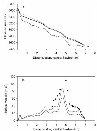
Fig. 6. Comparison between observed (dashed line/black dots) and modelled (solid lines) glacier elevation (a) and surface velocities (b) for AD 2000. The upper (lower) solid line corresponds to SOF (MAK) results.
