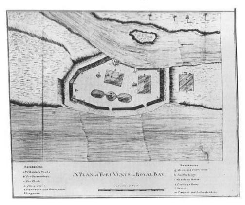
**Figure 2.** Plan of Fort Venus, Matavai Bay (after Parkinson 1784: Plate IV), showing the location of the circular tent observatory which housed the quadrant and journeyman clock, and the large rectangular tent with the astronomical clock.
