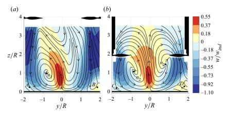
**Figure 4.** Time-averaged axial velocity contours and 2-D streamlines computed over one acquisition (2.7 s) for (a) H/R = 4 and (b) H/R = 2. Annotations  $n_1$ ,  $n_2$  and  $n_3$  denote nodal points in the domain.
