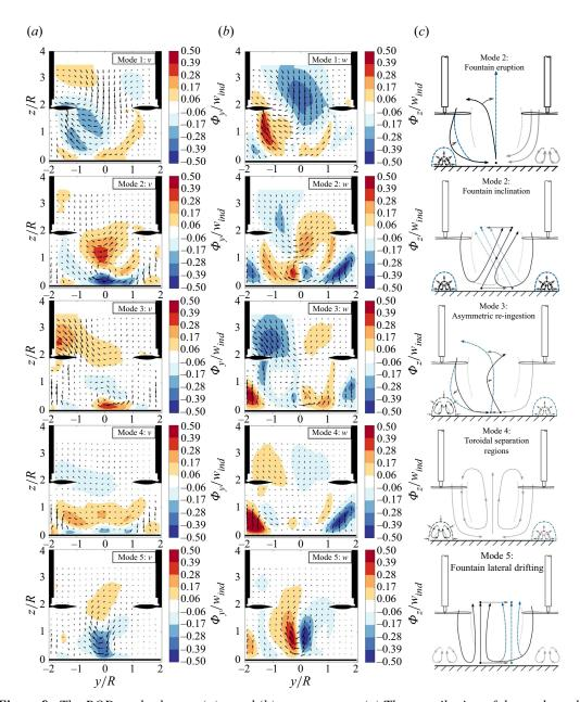
**Figure 9.** The POD mode shapes: (a) v and (b) w component. (c) The contribution of the mode to the flow field when the time coefficient decays from positive unity (black streamlines) to negative unity (blue streamlines).
