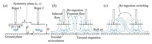
**Figure 1.** (a) Schematic representation of the side-by-side rotor system in ground effect with relevant parameters and system of coordinates. (b) Conceptual flow topology. (c) Illustration of re-ingestion switching.
