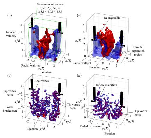
Figure 3. Iso-surfaces of normalized velocity magnitude  $V/w_{ind} = 0.5$  (blue) and  $w/w_{ind} = 0.25$  (red) for (a) H/R = 4 and (b) H/R = 2. Iso-surfaces of  $\lambda_2 = -60\,000\,\mathrm{s}^2$  (blue) and  $\lambda_2 = -90\,000\,\mathrm{s}^2$  (red) for (c) H/R = 4 and (d) H/R = 2. The measurement volume is illustrated by the green box in (a).
