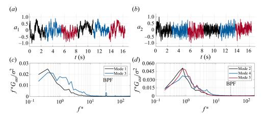
**Figure 10.** Temporal POD coefficient of (a) mode 1,  $a_1$ , and (b) mode 2,  $a_2$ . Pre-multiplied energy spectra of the temporal coefficients of (c) modes 1 and 3 and (d) modes 2, 4 and 5. The frequency has been normalized by the convective frequency, i.e.  $f^* = f/f_{conv}$ .
