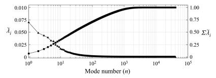
Figure 8. Energy fraction and cumulative energy as a function of POD mode number n.
