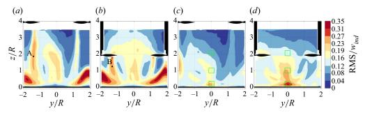
**Figure 5.** Root mean square of velocity fluctuation in axial direction for (a) H/R = 2 and (b) H/R = 4, and in lateral direction for (c) H/R = 2 and (d) H/R = 4. Green rectangles denote the regions where the vectors are extracted for generating figure 6.
