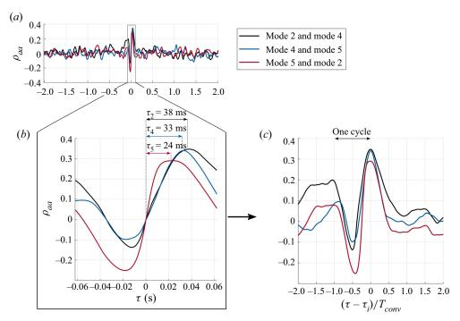
**Figure 12.** (a) Overview and (b) zoomed-in plot of the temporal cross-correlation coefficient, and corresponding lags for modes 2, 4 and 5. (c) Same as (a,b) but subtraction of lags in (b) and normalization of lag  $\tau$  by  $T_{conv}$ .
