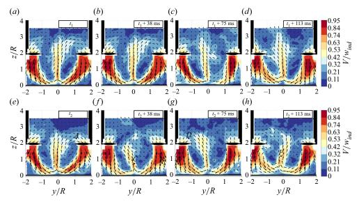
**Figure 7.** Normalized velocity magnitude contours  $V/w_{ind}$  and 2-D velocity vectors of two time sequences of sliding averages (ensembles of 100 samples/0.25 s), with a temporal increment of dt = 0.0375 s. The series (a-d) is statistically independent from the series (e-h), with  $t_2 = t_1 + 1.7$  s.
