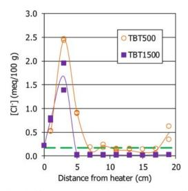
Fig. 6. Cl<sup>-</sup> concentration in the aqueous extracts of samples of the two TH tests and of the original material (dashed line).
