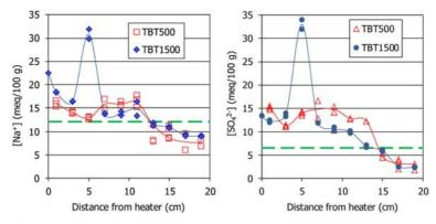
Fig. 5. Na and  $SO_4^{2-}$  concentrations in the aqueous extracts of samples of the two TH tests and of the original material (dashed lines).
