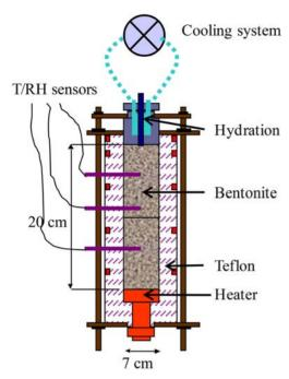
Fig. 1. Schematic design of the thermo-hydraulic cells.
