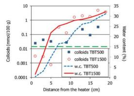
Fig. 16. Computed colloid concentration along the bentonite columns and in the original material (dashed line) and water content (w.c.) measured at the end of the tests.
