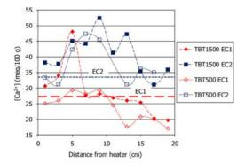
Fig. 15. Ca concentration in the exchange complex after the TH tests and in the original material (dashed lines), as determined with methods EC1 and EC2.
