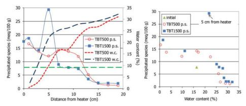
Fig. 17. Water content (w.c.) and ionic species precipitated (p.s.) along the columns estimated from the difference in ion content in the aqueous extracts and in the pore water. Dashed line: original amount of precipitated species.
