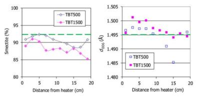
Fig. 3. Smectite content and  $d_{060}$  spacing along the columns and in the original material (dashed lines) as determined by XRD.
