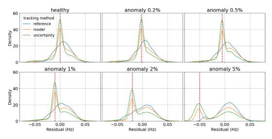
*Figure 11.* Residuals of three methods on a synthetic dataset with an increasing introduced anomaly on the physical mode with harmonic interaction.
