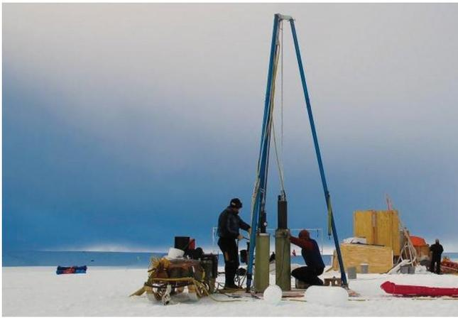
**Fig. 6.** The BID coring at the surface on Taylor Glacier. Notice the anti-torque handles attached to the outer barrel via a clamping device for near-surface coring. Photo by Robb Kulin.
