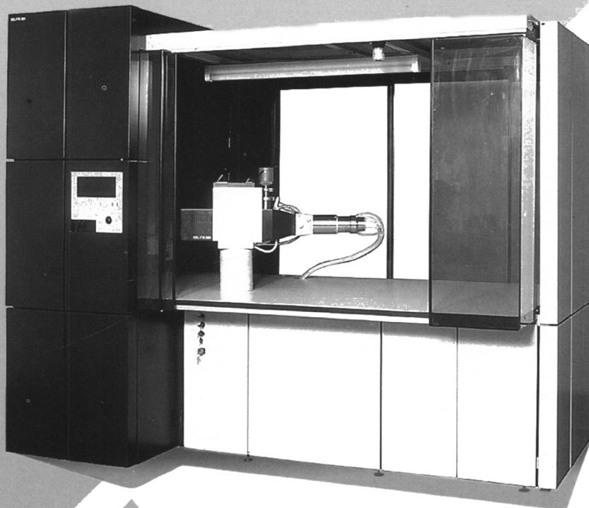
**Analytical and research scientists applying a strong laboratory X-ray source, need a powerful, easy to use, safe and very reliable rotating X-ray generator. Knowing this, NONIUS now offers: the <sup>NONIUS</sup> FR591 Rotating Anode X-ray Generator.**
